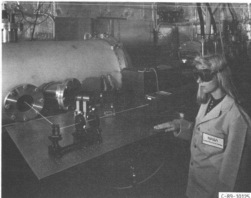
FIGURE 8. - RAMAN SPECTROSCOPY APPARATUS USING AN ARGON ION LASER.
