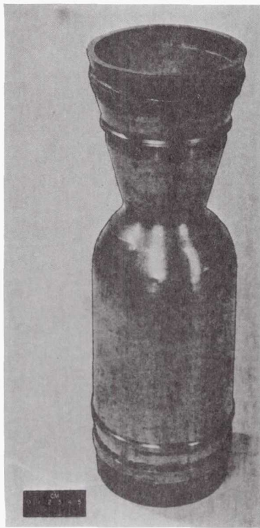
FIGURE 4. - MILLED COPPER LINER COMBUSTION CHAMBER WITH ELECTROFORMED NICKEL CLOSEOUT.
