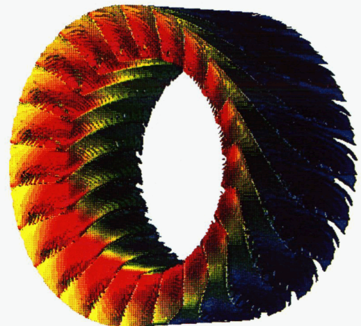
FIGURE 17. - MACH NUMBER CONTOURS FOR SWIRL VANE ASSEMBLY WITH TWIST.
