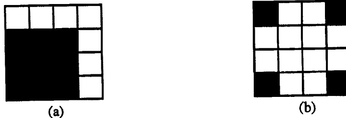
Figure 1. (a) Simple binary nine pixel image A, (b) the result of D_1 * A , the differential operator acting on A
