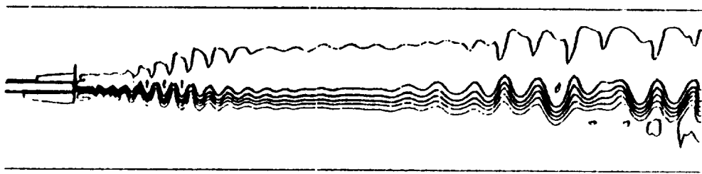
Figure 9. Temperature contours in mixing layer.
