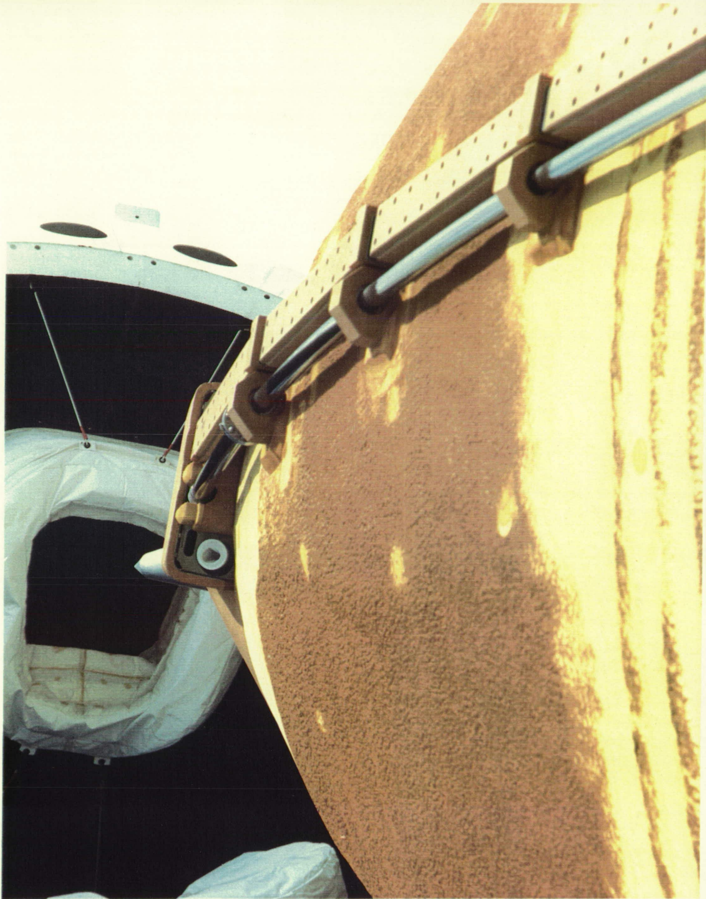
Prelaunch condition of ET tumble valve cover
