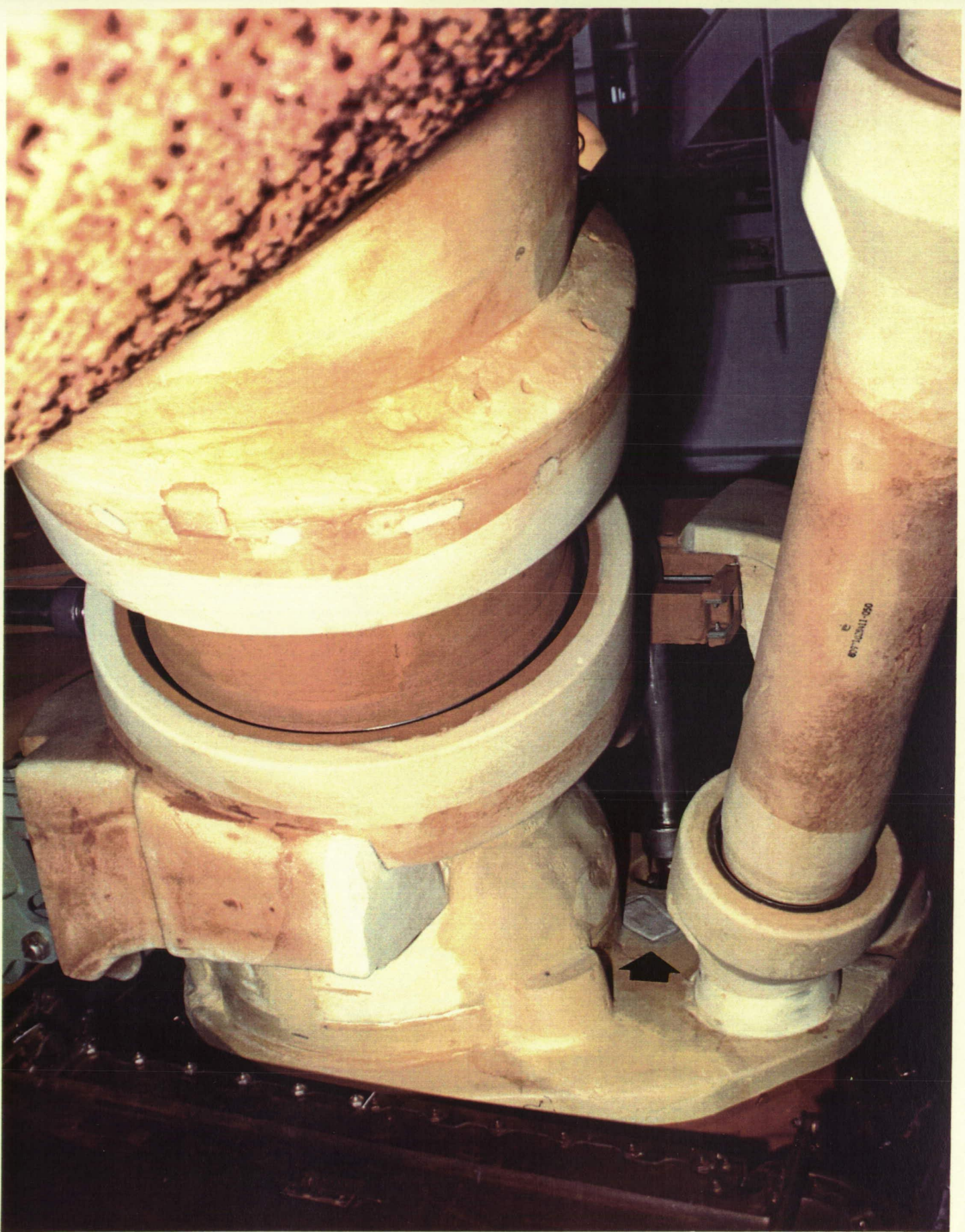
Overall view of LH2 ET/ORB umbilical. Note PDL foam plug in flapper valve actuator torque tool port closeout (arrow)
