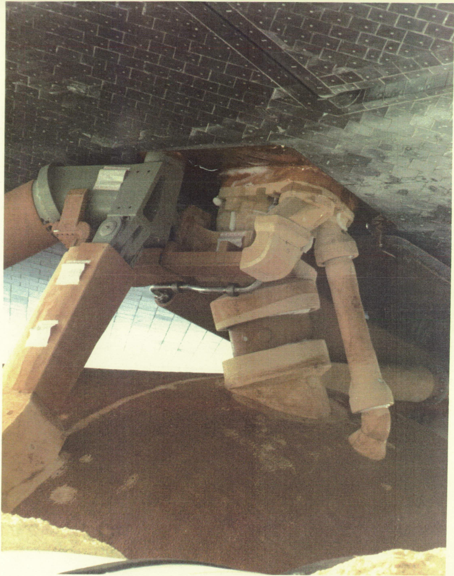
Hard ice is still present on the LH2 umbilical outboard side, purge vents, feedline and recirc line bellows after ET drain
