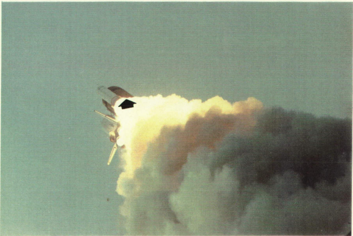
As many as 27 particles, most likely SRB aft skirt instafoam, fall from the vehicle just after the roll maneuver (E-59)
