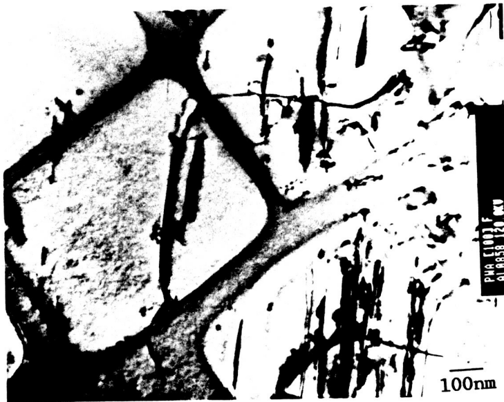
Figure 7. "V" shaped superdislocation.
