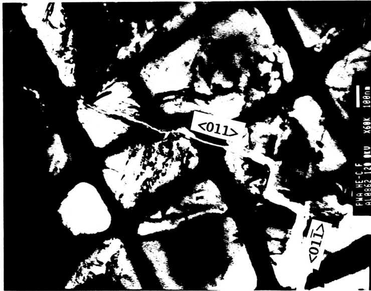
Figure 4. Cracking along \langle 011 \rangle and \langle 0\bar{1}\bar{1} \rangle directions on a (111) slip plane.
