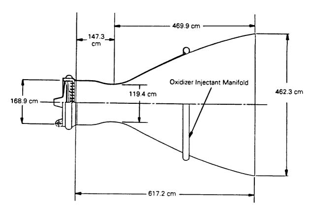
Figure 19. Single pass regeneratively cooled thrust chamber.
