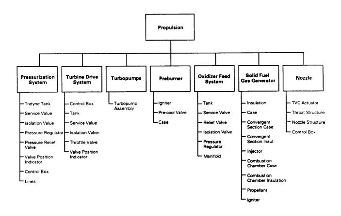
Figure 77. Hybrid propulsion system.
