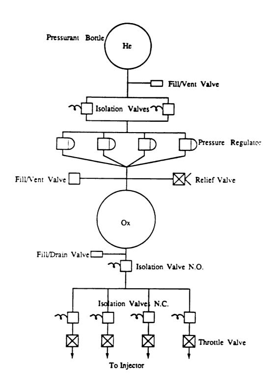
Figure A-4. Cold Gas Pressurization System Schematic for GG/LOX.
