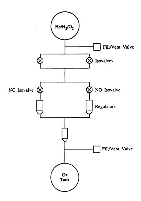
Figure A-16. Stored Reactive Gas (Tridyne) Pressurization System.
