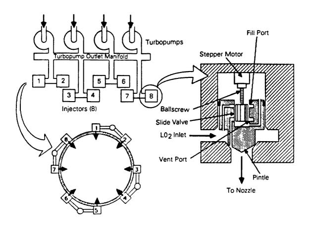
Figure 30. Hybrid booster program FITVC schematic.
