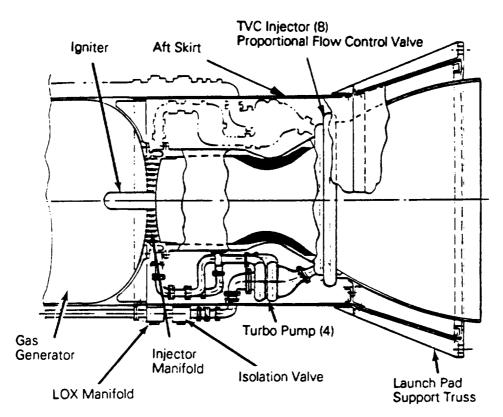
Figure 15. Thrust chamber design.
