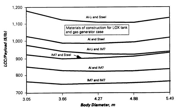
Figure 58. LCC/payload vs body diameter for the pump fed large booster.
