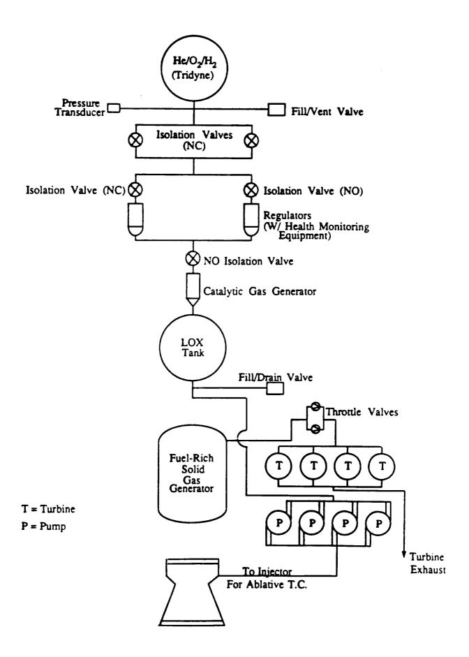
Figure A-17. <u>Preliminary Oxidizer Pump Fed System Schematic</u>.
