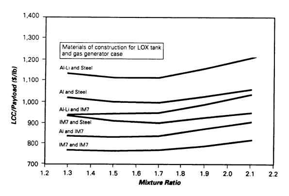
Figure 52. <u>Mixture ratio vs LCC/payload for the pump fed large booster.</u>
