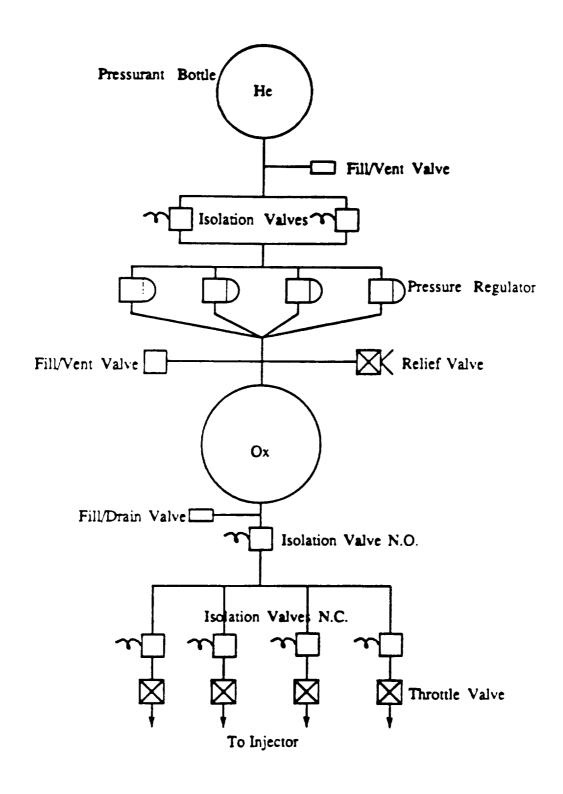
Figure A-1. Cold Gas Pressurization System Schematic.
