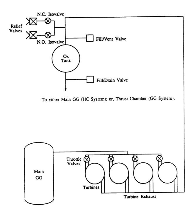
Figure A-15. <u>Autogeneous Pressurization System.</u>
