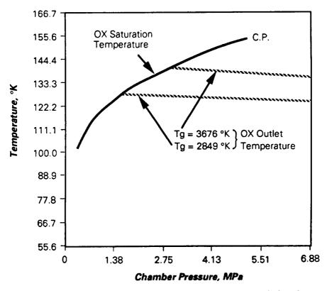
Figure 18. Relationship between coolant temperature and chamber pressure.
