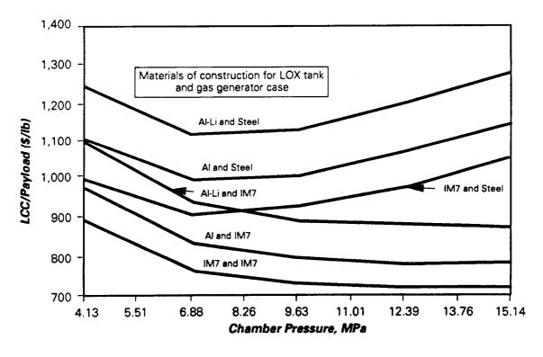
Figure 56. LCC/payload vs chamber pressure for the pump fed large booster.
