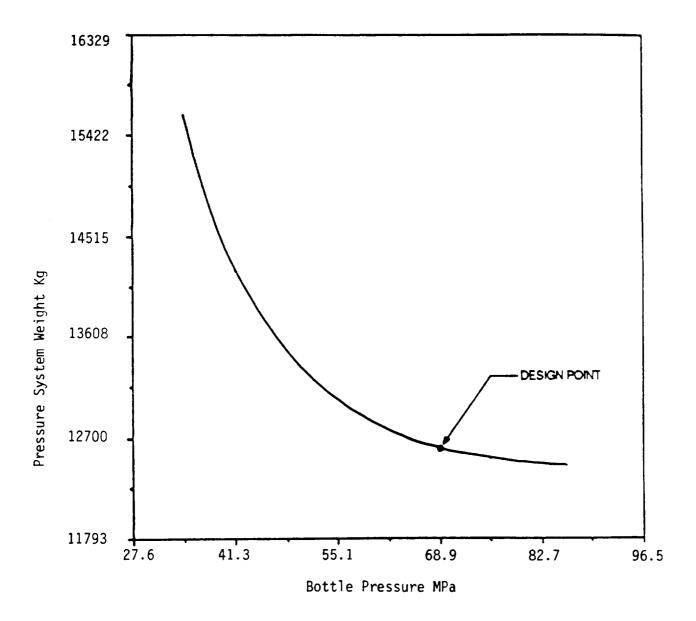
Figure 9. GG/LOX Hybrid System Weight vs Bottle Pressure.
