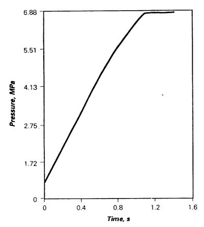
Figure 38. Predicted start-up pressure transient full-size booster.
