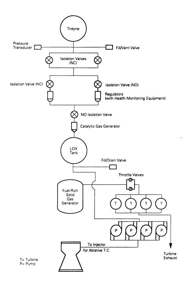
Figure 23. Preliminary oxidizer pump-fed system schematic.
