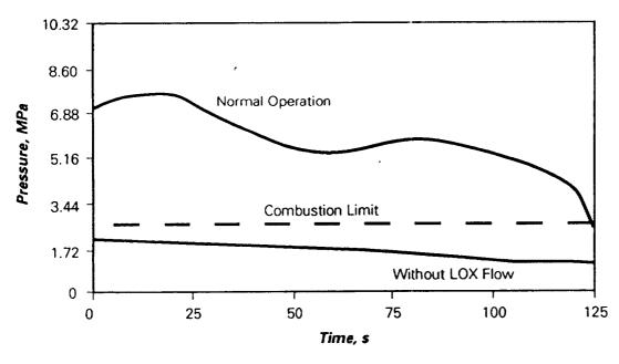
Figure 39. Gas generator pressure.
