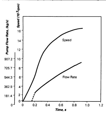
Figure 36. Turbopump start-up characteristics.
