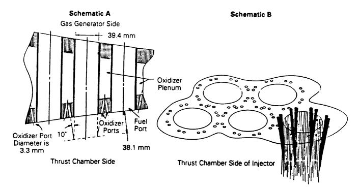
Figure 21. Injector manifold design.
