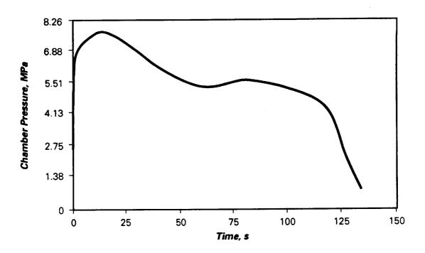
Figure 33. The predicted chamber pressure for the full-size booster grain design.
