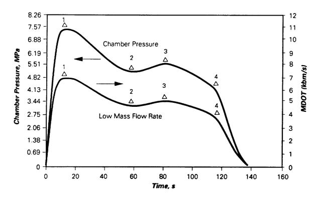
Figure 26. Selected turbopump operating points.
