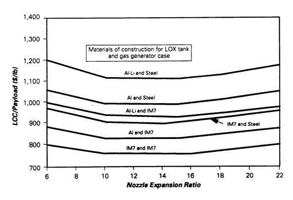
Figure 54. <u>LCC/payload vs expansion ratio for the pump fed large booster.</u>
