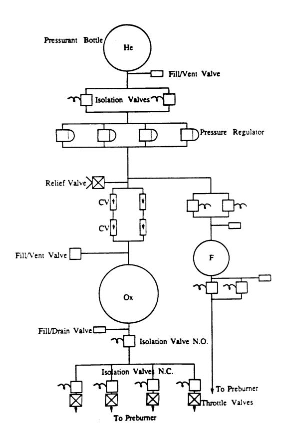
Figure A-5. Cold Gas Pressurization System Schematic for HC/LOX.
