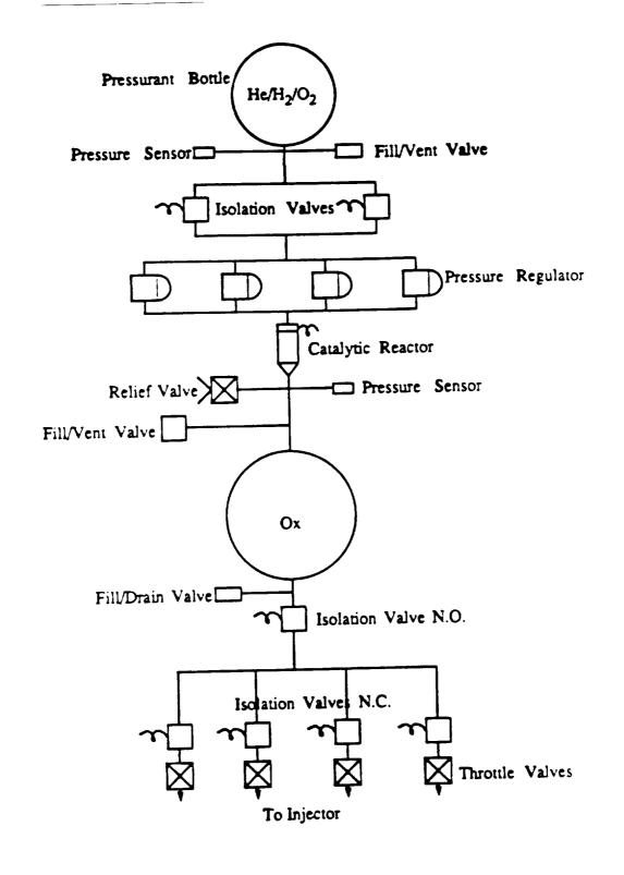
Figure A-8. Catalytic Warm Gas Pressurization System Schematic for GG/LOX.
