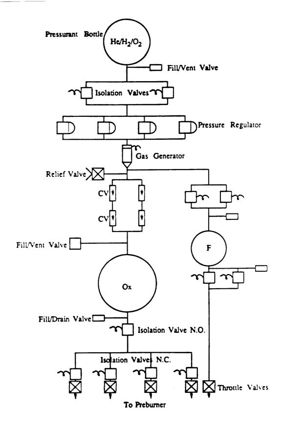
Figure A-7. Catalytic Warm Gas Pressurization System Schematic for HC/LOX.
