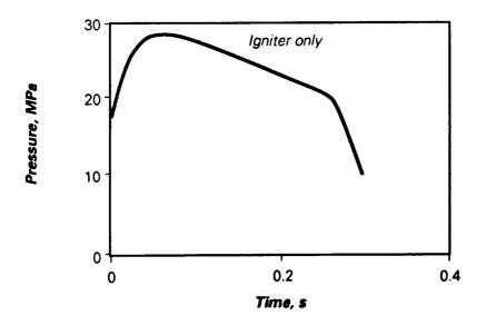
Figure 14. Igniter pressure traces (full-size booster).
