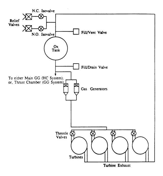
Figure A-13. <u>Autogeneous Pressurization System</u>.
