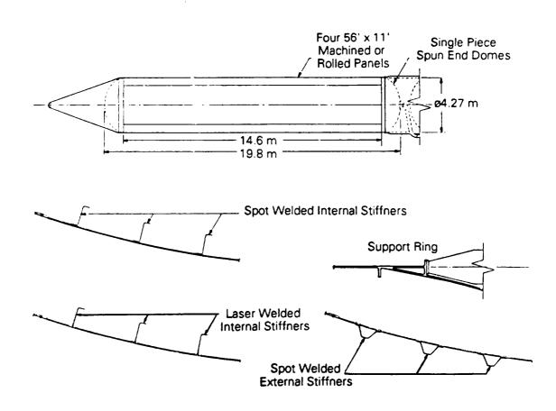
Figure 27. Aluminum-lithium LOX tank design.
