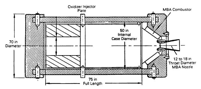
Figure 82. 50 in heavywall subscale demonstrator motor.
