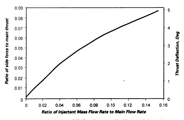
Figure 29. Hybrid engine FITVC performance (liquid oxygen injectant).
