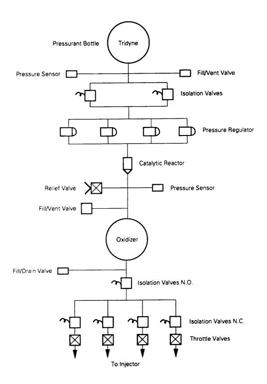
Figure 22. Catalytic warm gas pressurization system schematic for GG/LOX.
