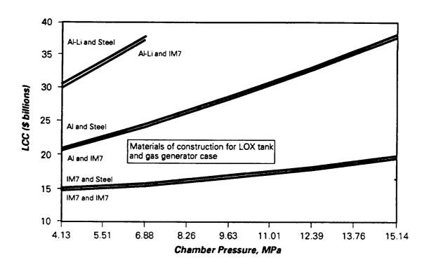
Figure 63. LCC vs chamber pressure for the pressure fed large booster.
