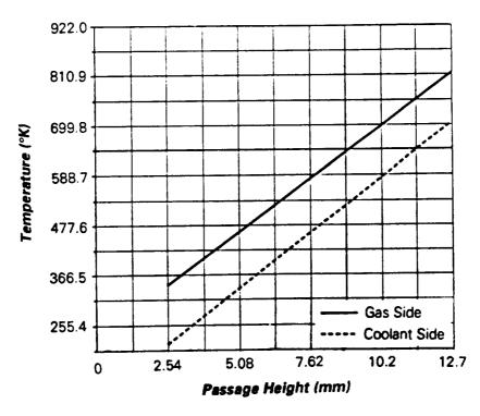
Figure 16. Throat wall temperature as a function of passage height.
