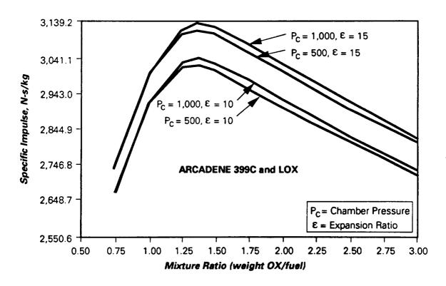
Figure 10. <u>Vacuum I<sub>SP</sub> versus mixture ratio, expansion ratio, and chamber pressure.</u>
