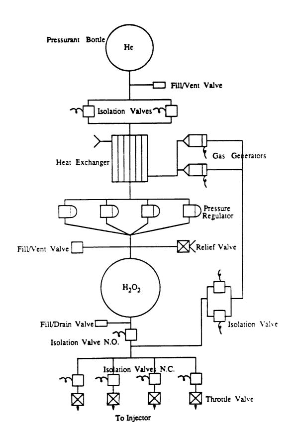
Figure A-3. <u>Cold Gas With Gas Generator/Heat Exchanger</u>
