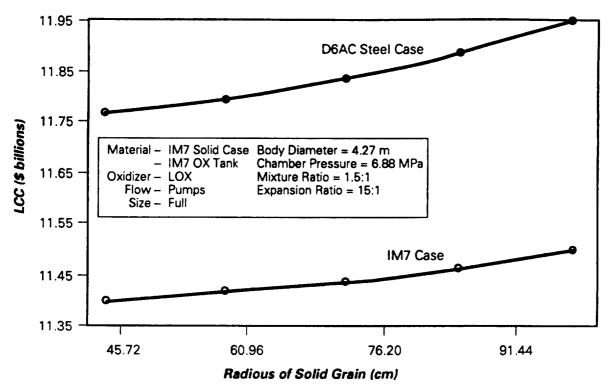
Figure 74. Life cycle cost vs grain radius.
