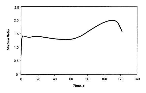
Figure 45. Quarter-size booster mixture ratio.
