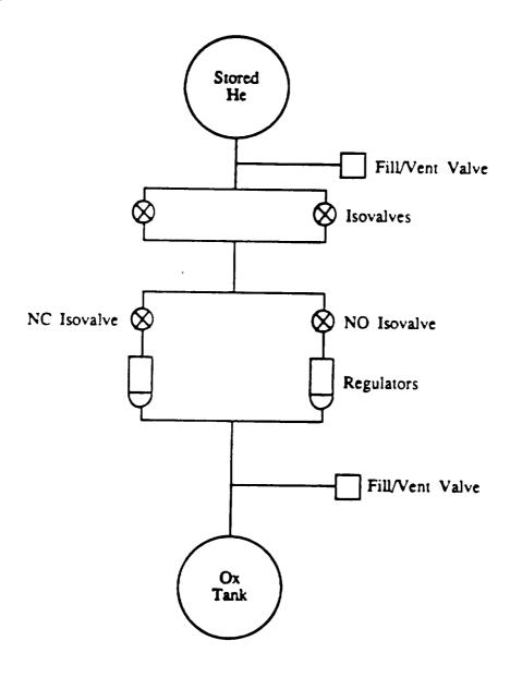
Figure A-12. Stored Helium Gas Pressurization System.
