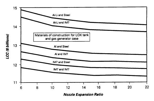
Figure 53. LCC vs expansion ratio for the pump fed large booster.
