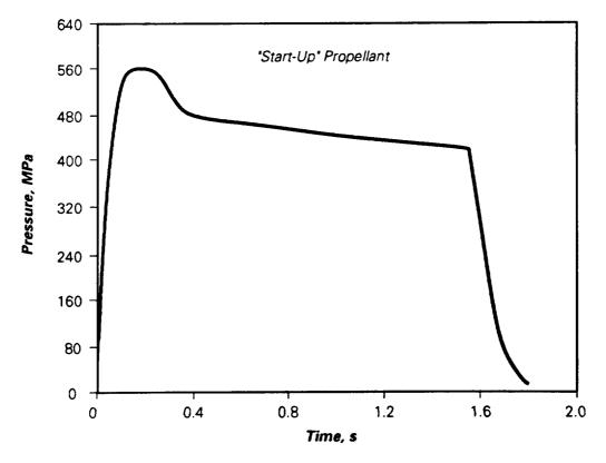
Figure 12. Igniter Pressure traces for full-size booster.
