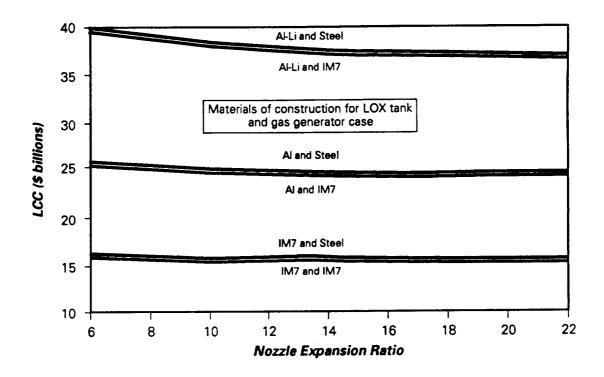
Figure 61. LCC vs expansion ratio for the pressure fed large booster.
