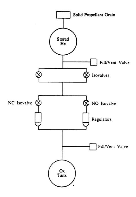
Figure A-14. Stored Gas (Solid Grain Augmented).
