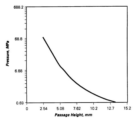
Figure 17. Coolant passage pressure drop as a function of passage height.
