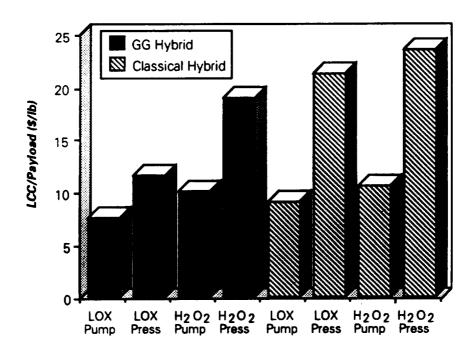
Figure 49. Hybrid concept comparison. LCC/payload.
