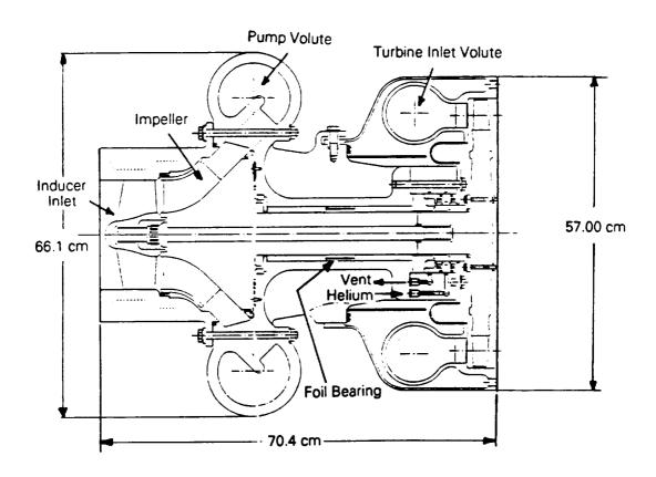
Figure 25. LOX turbopump.
