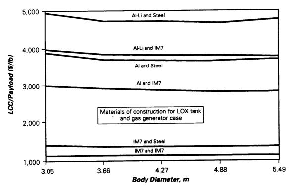
Figure 66. LCC/payload vs body diameter for the pressure fed large booster.
