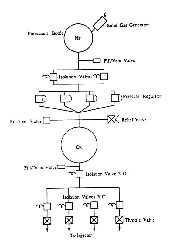
Figure A-2. Warm Gas Pressurization System Schematic.
