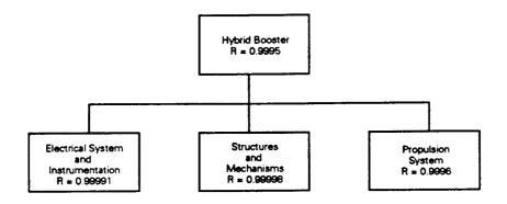
Figure 76. Hybrid booster reliability block diagram.
