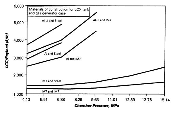
Figure 64. <u>LCC/payload vs chamber pressure for the pressure fed large booster</u>.
