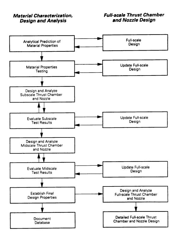
Figure 80. Full-scale nozzle design activity interacts with material characterization, design, technology efforts.
