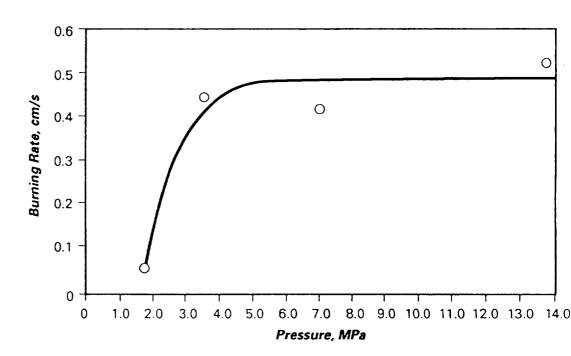
Figure 40. Burning rate vs pressure.
