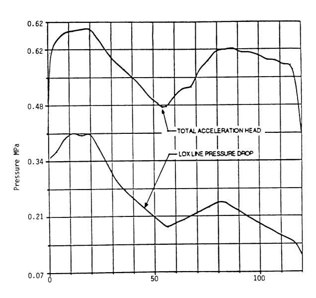
Figure A-10. GG/LOX Hybrid Acceleration Head and LOX Line Pressure Drop.
