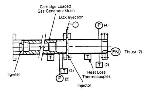
Typical 22.9 cm (9 in) Test Set-up
