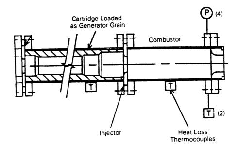
Typical 7.6 cm (3 in) Test Set-up
