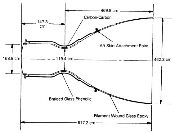
Figure 20. Ablative thrust chamber design.
