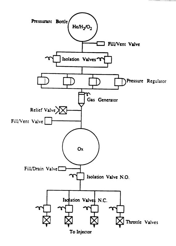
Figure A-6. Catalytic Warm Gas Pressurization System Schematic for GG/LOX.
