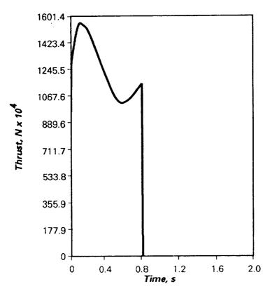
Figure 41. Emergency shutdown thrust.
