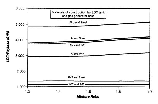
Figure 60. <u>Mixture ratio vs LCC/payload for the pressure fed large booster.</u>
