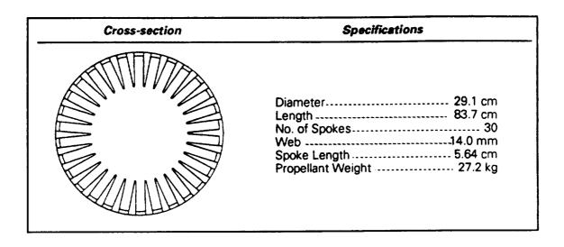
Figure 13. Igniter grain design (full-size booster).
