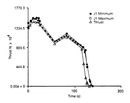
Figure 32. Predicted thrust trace full-size booster.
