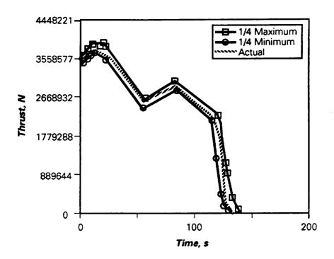
Figure 44. Quarter-size booster thrust trace.
