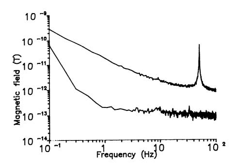
In fig.3 the ambient noise spectrum is depicted (upper curve), which was read at night at a distance of 20m from the nearest Laboratory building in Dubna. It is clearly seen, that the ambient noise is considerably higher than the squid self-noise. Thus, we can suppose that such a magnetometer can be used for geophysical investigations.
