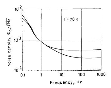
easily obtain the estimate of the squid field sensitivity: ${}^{<}B_N^{>}={}^{<}\phi_N^{>}B_O^{/}\phi_O^{}$ , where  ${}^{<}\phi_N^{>}$  - squid spectral noise density on magnetic flux.
