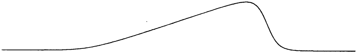
Figure 1.7. Solution to the viscous Burgers' equation at time T_b for the data shown in Figure 1.5.
