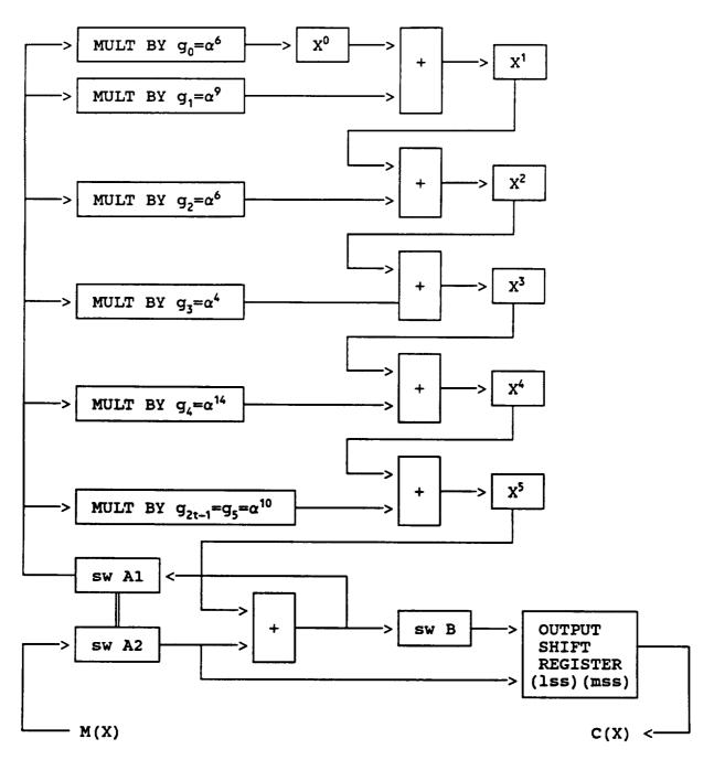
Figure A.1-1. - (15,9) RS encoder shift register circuit.
