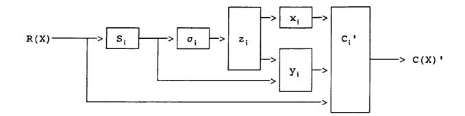
Figure B.4-2. - High data rate RS pipelined decoder.
