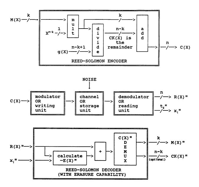
Figure 5.1-1. - RS coding block diagram with erasure capability.
