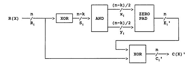
Figure B-1. - Combinational RS decoding circuit.
