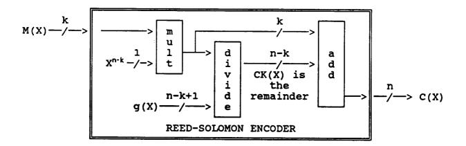
Figure 3.1-1. - Block diagram of a Reed-Solomon encoder.
