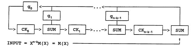
Figure A.2-1. - Encoder SRC using  $CK(X) = M(X) \mod q(X)$ .
