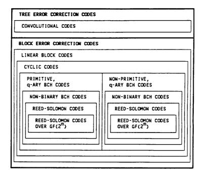
Figure 2.3-1. - General Venn diagram of error correction codes.
