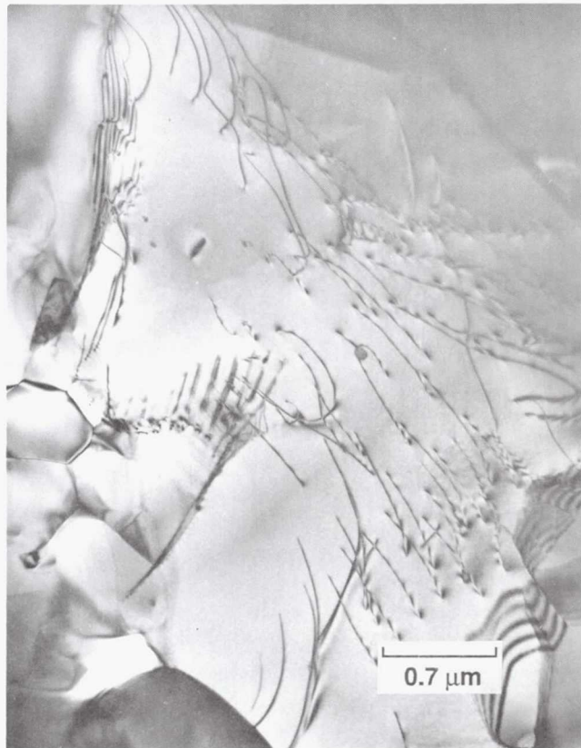
Figure 8.—Dislocations in deformed \text{Si}_3\text{N}_4\text{-Sc}_2\text{O}_3 , having Burgers vector of [0001] .
