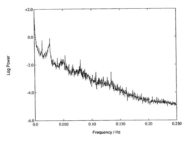
24. Power spectrum of the velocity **u** at  $\Omega = 12.5\Omega_c$ . The driving frequency and its subharmonics are still dominant in the spectrum. . . . . .
