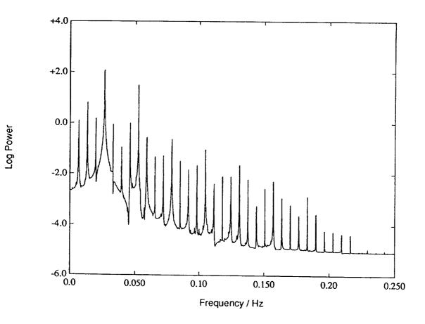
17. Power spectrum of the velocity u at  $\Omega = 9.458\Omega_c$ . Two period-doublings have taken place.
