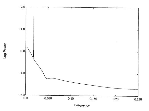
16. Power spectrum of the velocity **u** at  $\Omega = 5\Omega_c$ . Only one frequency present in the problem.
