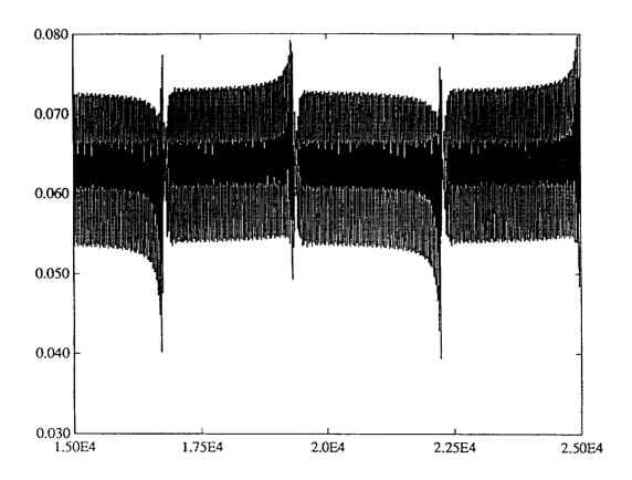
8. a) Time series of  $Re(u_{(0,1)})(t)$  at  $\Omega = 4.48\Omega_c$ . The flow is intermittent chaotic with long time intervals between the bursts of activity.
