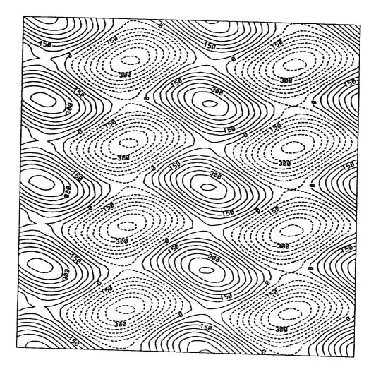
4. Steady cellular flow found at  $\Omega = 2\Omega_c$  with the motion mainly in vertical direction and the fastest growing perturbation with wavenumber 2 in horizontal direction. a) streamlines.
