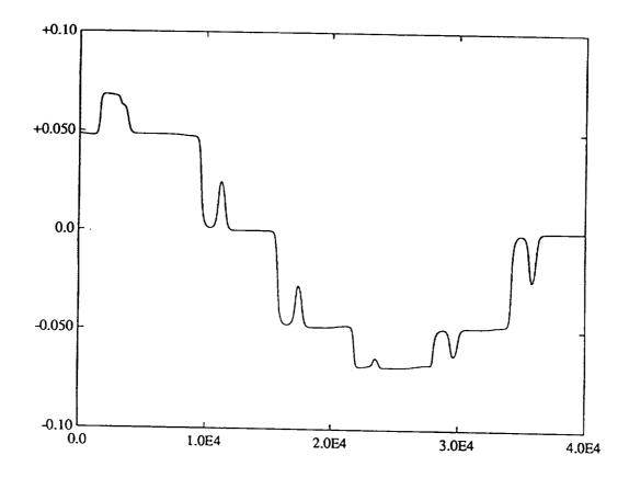
6. Time series of  $Re(u_{(0,1)})(t)$  at  $\Omega = 3.56\Omega_c$ . Plateaus correspond to a steady cellular flow.
