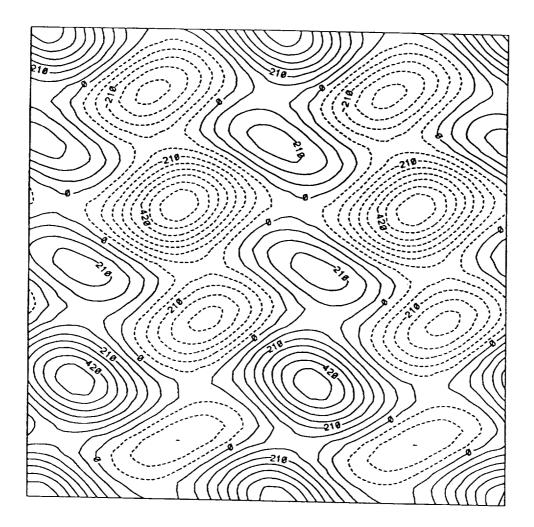
5. Steady cellular flow found at  $\Omega = 3\Omega_c$ . a) streamlines.
