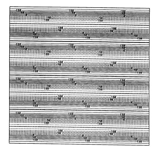
1. Parallel shear layer flow corresponding to the fixed point solution at  $\Omega = 0.5\Omega_c$ . a) streamlines.
