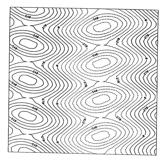
3. Steady cellular flow found at  $\Omega = 1.5\Omega_c$  with the motion mainly in vertical direction and the fastest growing perturbation with wavenumber 1 in horizontal direction. a) streamlines.
