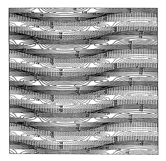
3. Steady cellular flow found at  $\Omega = 1.5\Omega_c$  with the motion mainly in vertical direction and the fastest growing perturbation with wavenumber 1 in horizontal direction. b)vorticity.
