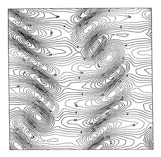
15. Steady spatially chaotic flow found at  $\Omega = 5.9\Omega_c$ . b) vorticity. Also, this is an example of large scale structures.
