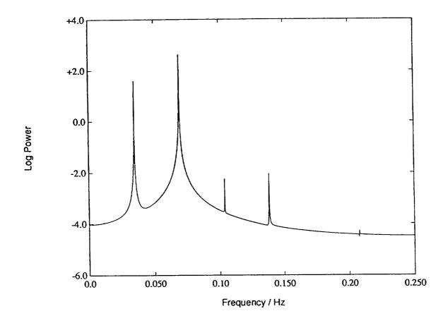
7. Power spectrum of the velocity **u** at  $\Omega = 4\Omega_c$ . The principal frequency and its subharmonic dominates the spectrum.
