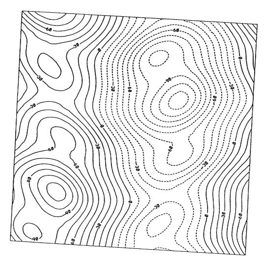
15. Steady spatially chaotic flow found at  $\Omega = 5.9\Omega_c$ . a) streamlines. Also, this is an example of large scale structures.
