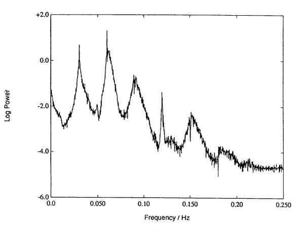
9. Power spectrum of the velocity **u** at  $\Omega = 4.48\Omega_c$ . The flow is chaotic, but the principal frequency and its subharmonics still dominate the spectrum.
