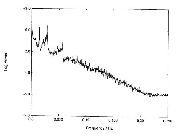
22. Power spectrum of the velocity **u** at  $\Omega = 10.805\Omega_c$ . The flow is chaotic, but the driving frequency and its subharmonics are dominant in the spectrum.
