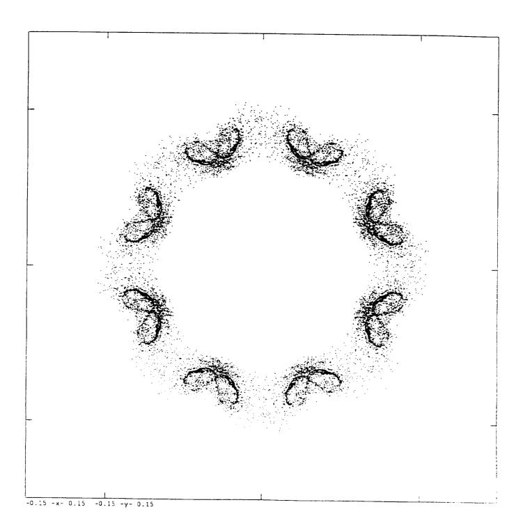
13. a) Poincare section of the chaotic attractor at  $\Omega = 4.63\Omega_c$ . Flow intermittently jumps from one component of the attractor to another.
