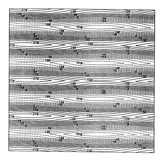
2. Steady cellular flow found at  $\Omega = 1.12\Omega_c$  with the motion mainly in horizontal direction. a) streamlines.
