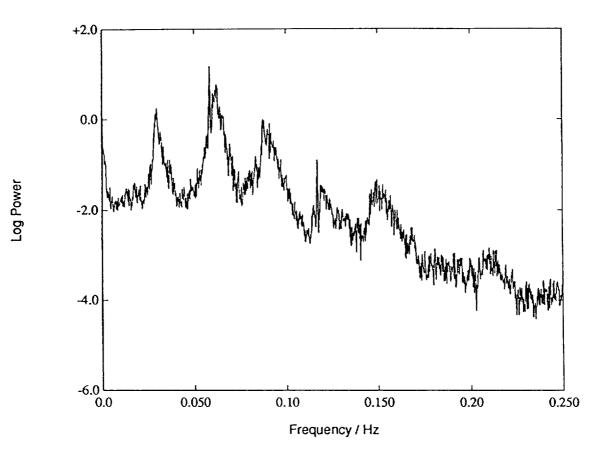
12. Power spectrum of the velocity **u** at  $\Omega = 4.63\Omega_c$ .
