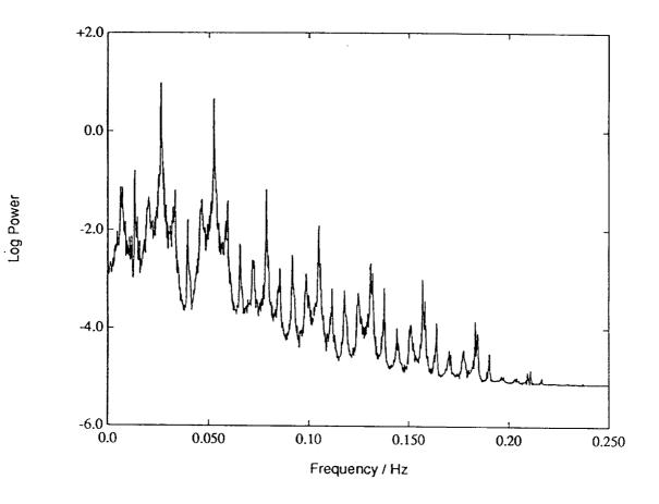
18. Power spectrum of the velocity **u** at  $\Omega = 9.47\Omega_c$ . The flow is chaotic, but the driving frequency and its subharmonics are still dominant in the spectrum.
