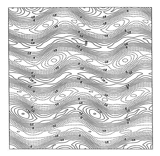
5. Steady cellular flow found at  $\Omega = 3\Omega_c$ . b) vorticity.
