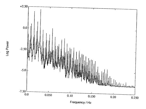
21. Power spectrum of the velocity **u** at  $\Omega = 10.7\Omega_c$ . One period-doubling have taken place in the range  $9.65 \leq \Omega/\Omega_c \leq 10.7$ .
