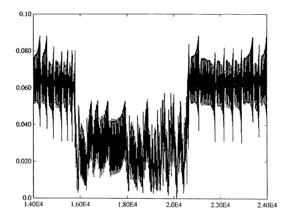
11. a) Time series of  $Re(u_{(0,1)})(t)$  at  $\Omega = 4.63\Omega_c$ . The flow is intermittent chaotic. The sudden jumps correspond to the solution jumping from one component of the chaotic attractor to another.
