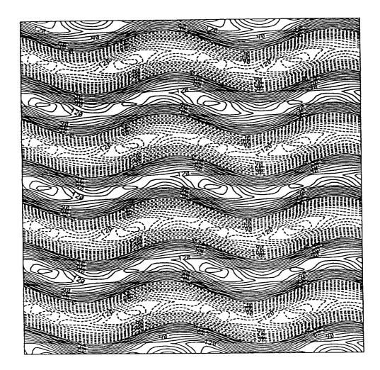
4. Steady cellular flow found at  $\Omega = 2\Omega_c$  with the motion mainly in vertical direction and the fastest growing perturbation with wavenumber 2 in horizontal direction. b) vorticity.
