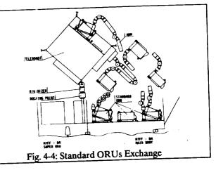
For this reason this figure must be seen in a general sense: it has been considered one non standard ORU of 350 Kg. (5 times the maximum standard ORU mass), with a height which does not interfere with the cover, and with the other dimensions proportional to the standard ORU ones. Within this data range it is possible to get a reasonable feeling of mission feasibility.
