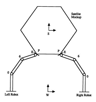
Figure 3: Coordinate Frame Assignments
