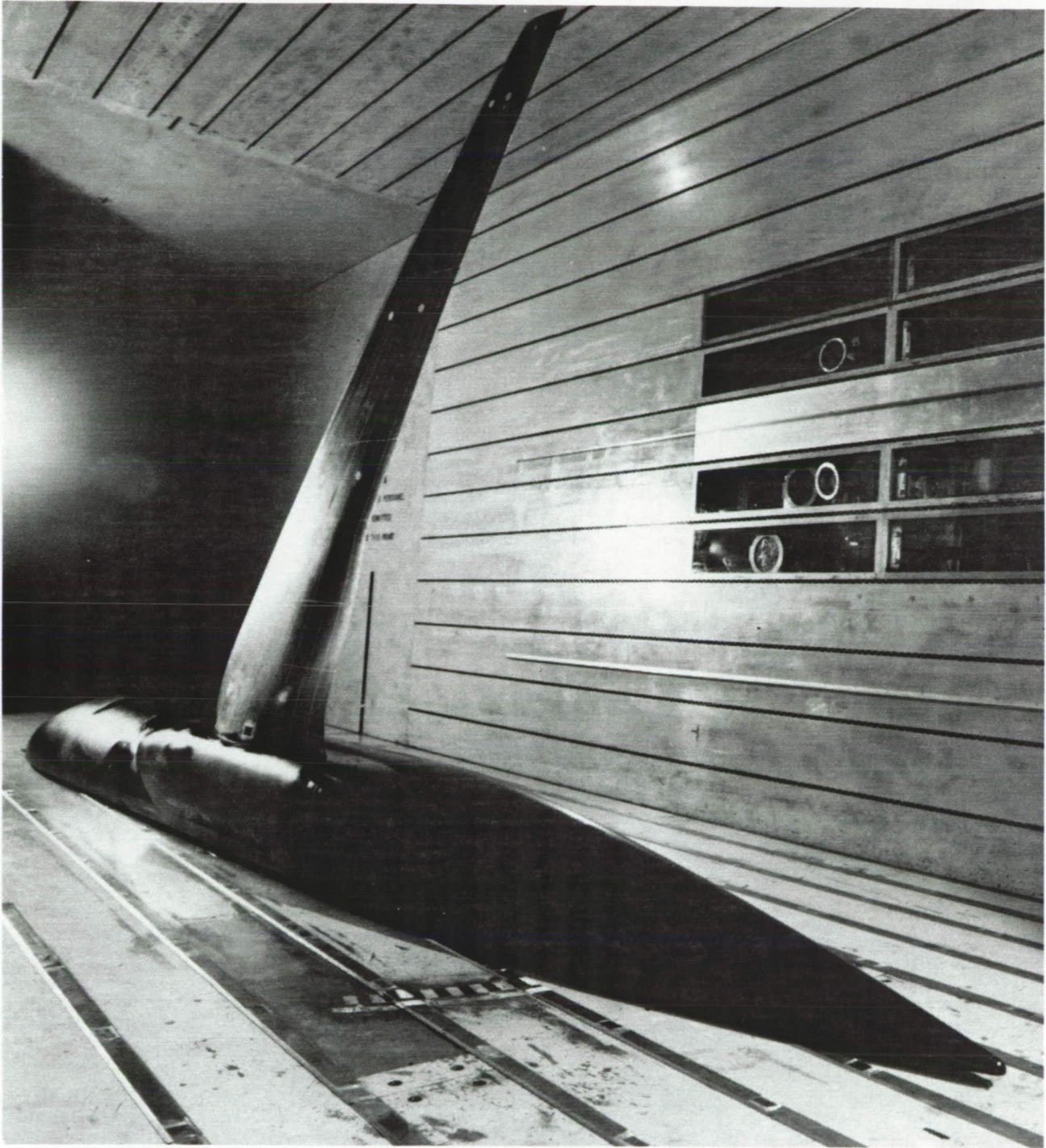
Fig. 2. Semispan model in the NASA Ames 11-Foot Transonic Wind Tunnel (installation photograph).
