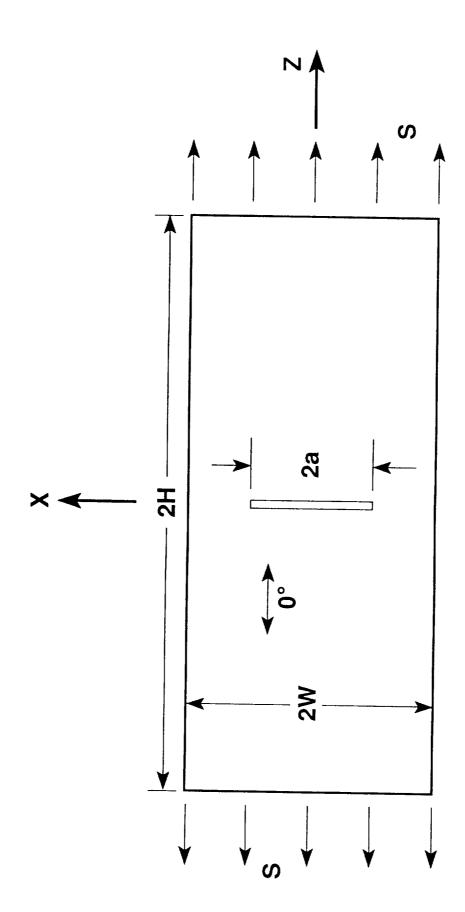
Figure 1. - Specimen geometry and loading. 2a = 19 mm, 2W = 78 mm, and  $2H = 101 \text{ mm}, v_f = 0.30.$
