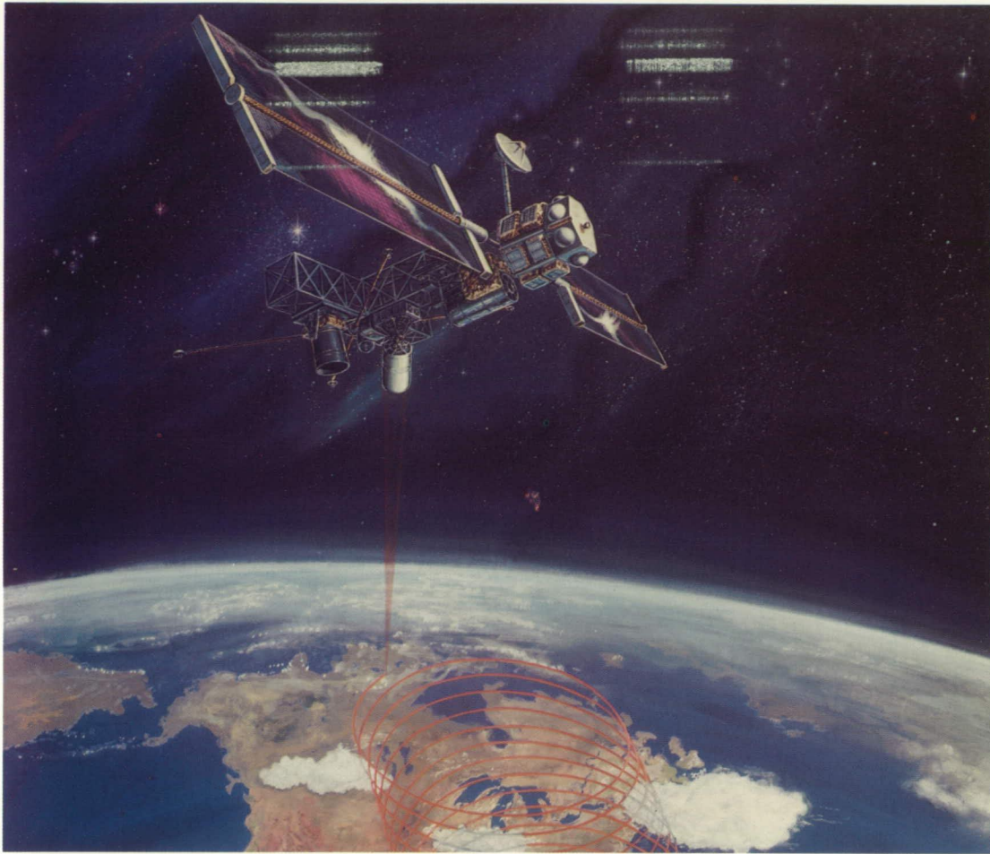
Laser Atmospheric Wind Sounder (LAWS)
