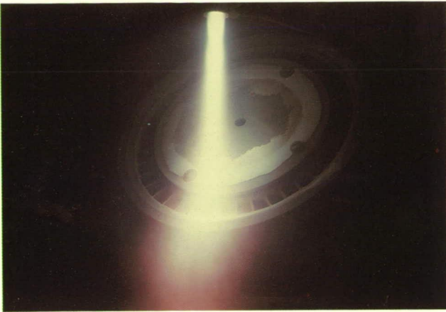
Vacuum Plasma Spray (VPS) application of a zirconia/nicaloy thermal-barrier coating on an SSME turbine component
