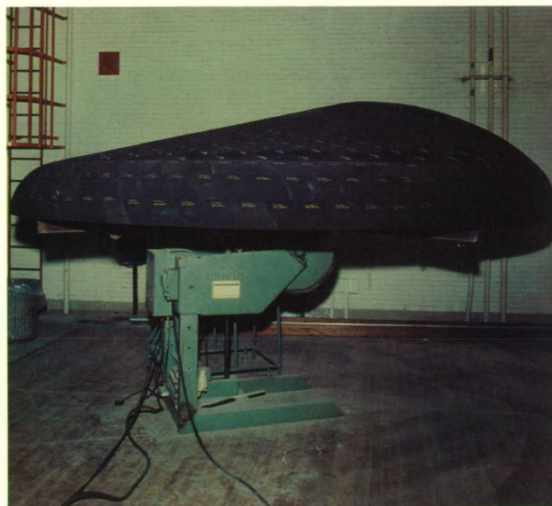
Heat shield (Shuttle Tile) installed on aerobrace mockup
