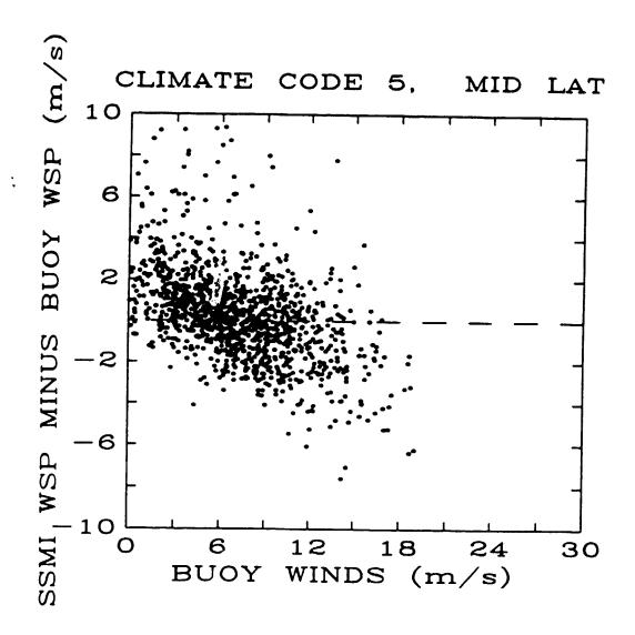
Figure 9. D-matrix residual plotted as a function of the coincident buoy winds for climate code 5.
