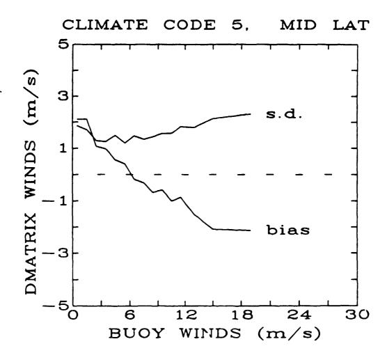
Figure 10. Standard deviation and bias of the D-matrix retrieved winds plotted as a function of buoy wind speed for climate code 5.
