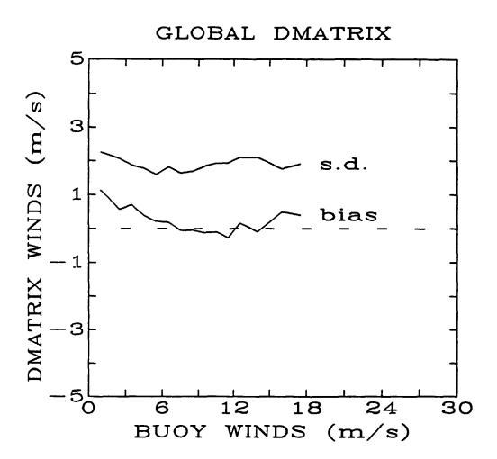
Figure 13. Standard deviation and bias of the global D-matrix retrieved winds plotted as a function of buoy wind speed.
