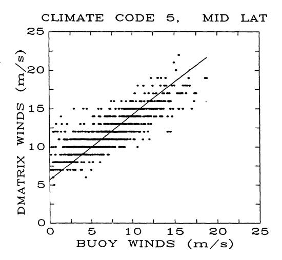
Figure 3. Performance of the original D-matrix algorithm for climate code 5. Bias = 5.7 m/s, slope = 0.85, S.D. = 5.1 m/s, corr (R) = 0.82, # obs = 998.
