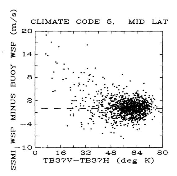
Figure 5. D-matrix residual plotted as a function of the rain-flag, (TB37V-TB37H), for climate code 5.
