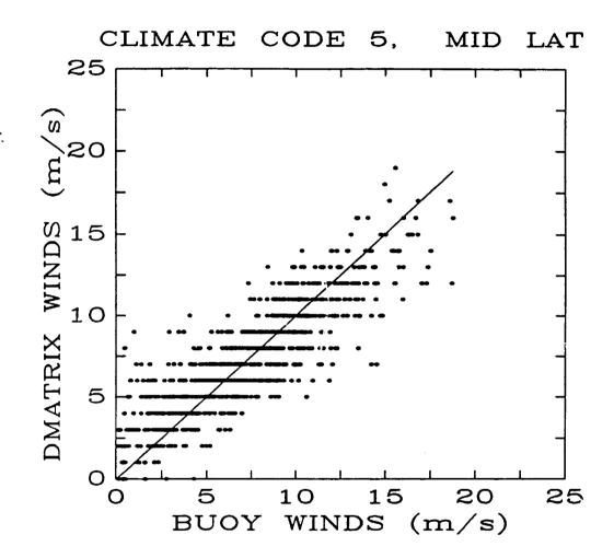
Figure 4. Performance of the revised D-matrix algorithm for climate code 5. Bias = 0.0 m/s, slope = 1.0 m/s, S.D. = 1.9 m/s, corr (R) = 0.85, # obs = 998.
