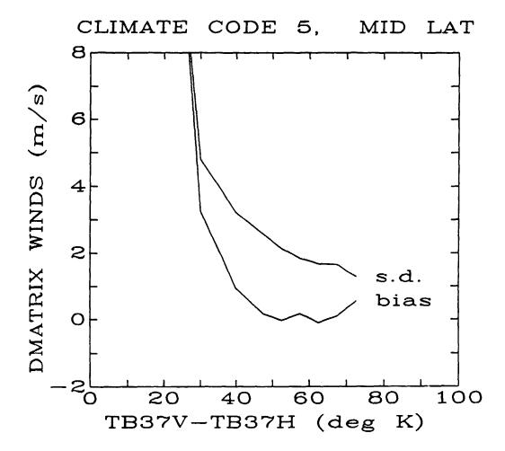
Figure 7. Standard deviation and bias of the D-matrix retrieved winds plotted as a function of the rain-flag. (TB37V - TB37H), for climate code 5.
