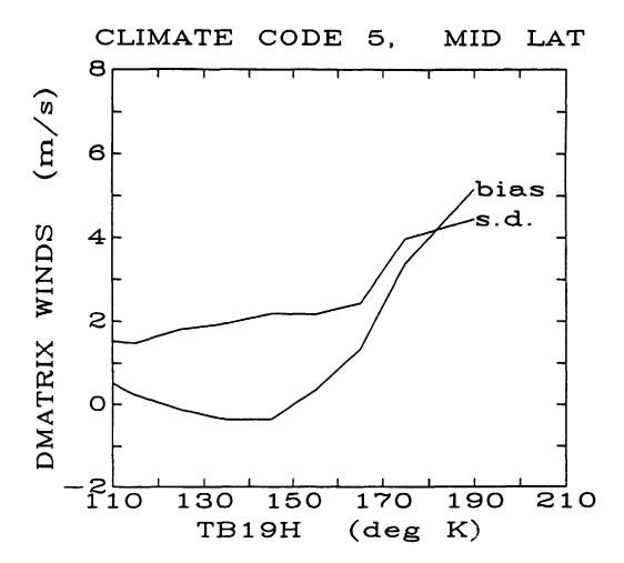
Figure 8. Standard deviation and bias of the D-matrix retrieved winds plotted as a function of the rain-flag, TB19H, for climate code 5.
