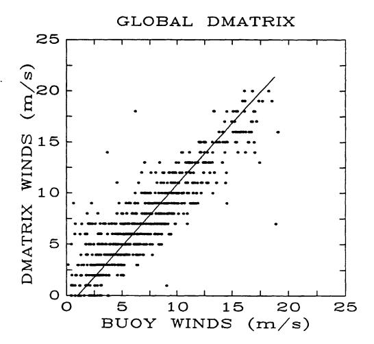
Figure 12. Performance of the global D-matrix algorithm. Bias = -1.1 m/s, slope = 1.2, S.D. = 2.0 m/s. corr (R) = 0.88, # obs = 708.
