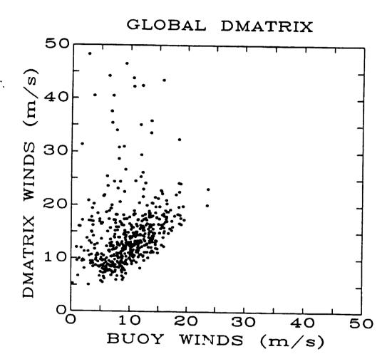
Figure 16. Performance of the global D-matrix algorithm under rain-flag 1, 2, and 3 conditions. S.D. = 8.0 m/s, corr (R) = 0.27, # obs = 525.
