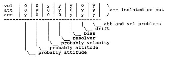
note: acc means either acc-x, acc-y, or acc-z 0 means O.K., y means yes there is a problem (i.e., an IMU miscompared with both other IMU's).
