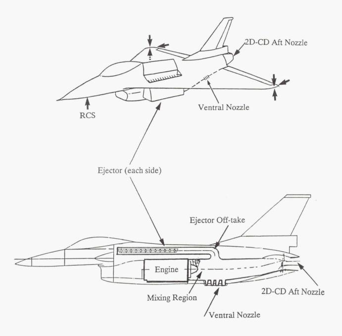
Fig. 1 E-7D/Ejector configured aircraft.
