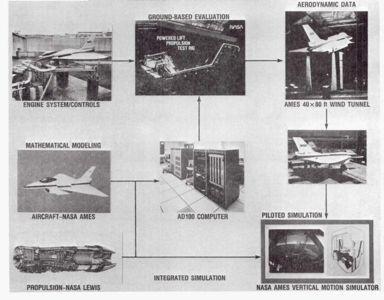
Figure 2. Integrated Controls Research Facilities
