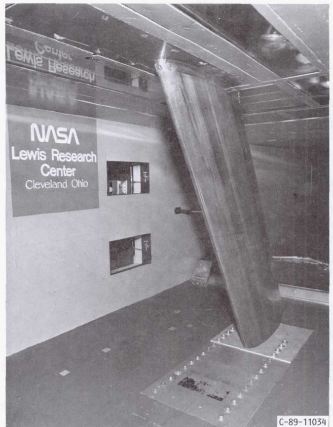
FIGURE 5. - MS-317 SWEEP WING MODEL USED TO OBTAIN ICE SHAPE TRACINGS.
