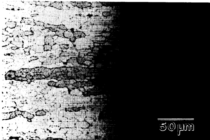
Figure 3 b. Optical micrograph of a large pit showing continuous subgrain boundary corrosion.
