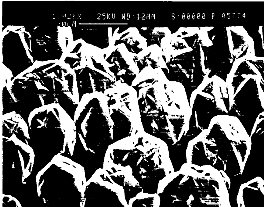
Fig. 5(b). SEM photograph of diamond crystallites on a carbide substrate.
