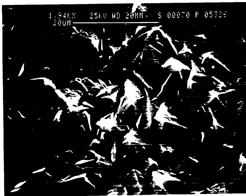
Fig. 5(a). Diamond film on Si substrate for 16 hours.
