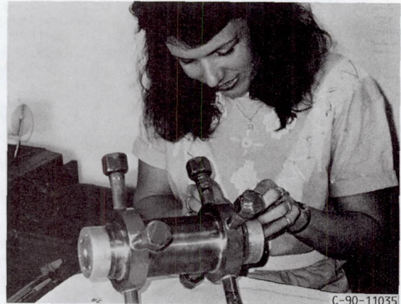
FIGURE 9. - PHOTOGRAPH OF TUBE ASSEMBLY WITH PREFABRICATED MANIFOLD INSERTS INSTALLED.
