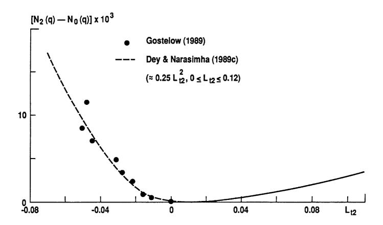
Figure 3. A preliminary proposal for the variation of the differential spot formation rate parameter  $N_2$  at the location of the subtransition point, at any given value of the free-stream turbulence level q, as a function of the Thwaites pressure gradient parameter at subtransition (from Narasimha and Dey 1989).
