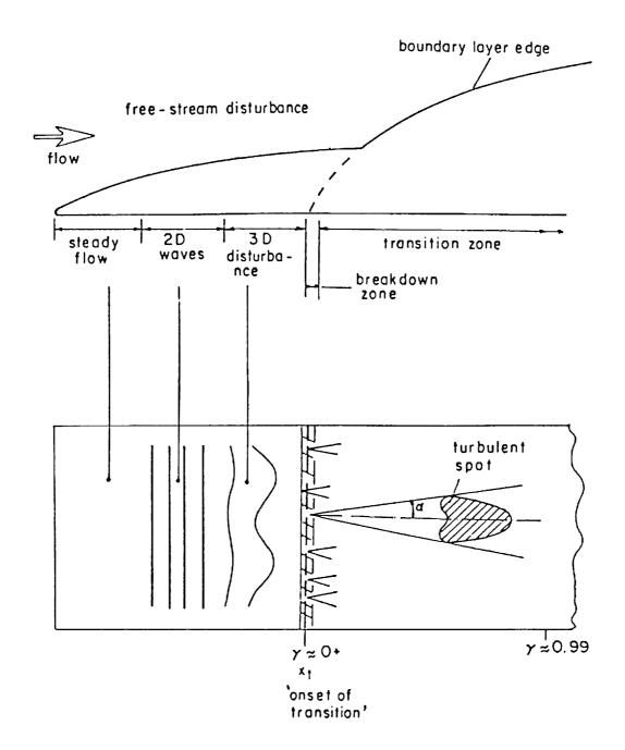
Figure 1. A schematic picture of various stages in the transition from laminar to turbulent flow in a flat plate.  $\alpha$  and  $\gamma$  respectively denote the spot spread angle and intermittency. The route shown here, one among many that are possible, seems to be relevant when external disturbances are low. The instability stages may be bypassed when the environment is highly disturbed.
