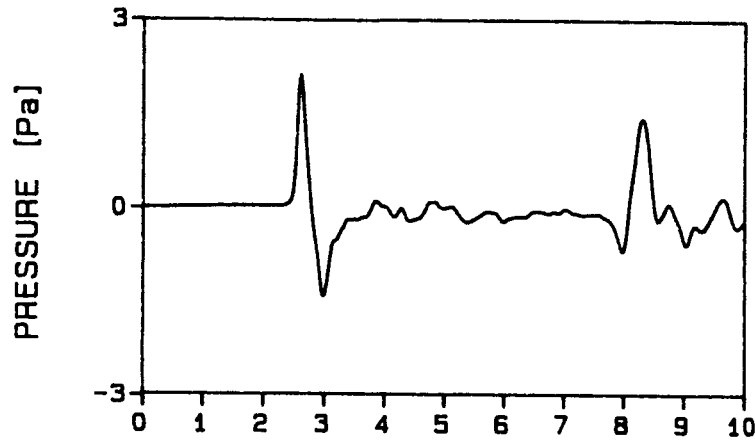
Fig. 3 a: Measured time signal h_s = h_r = 12.5 \text{ m} ; distance: 250 m (stable conditions)
