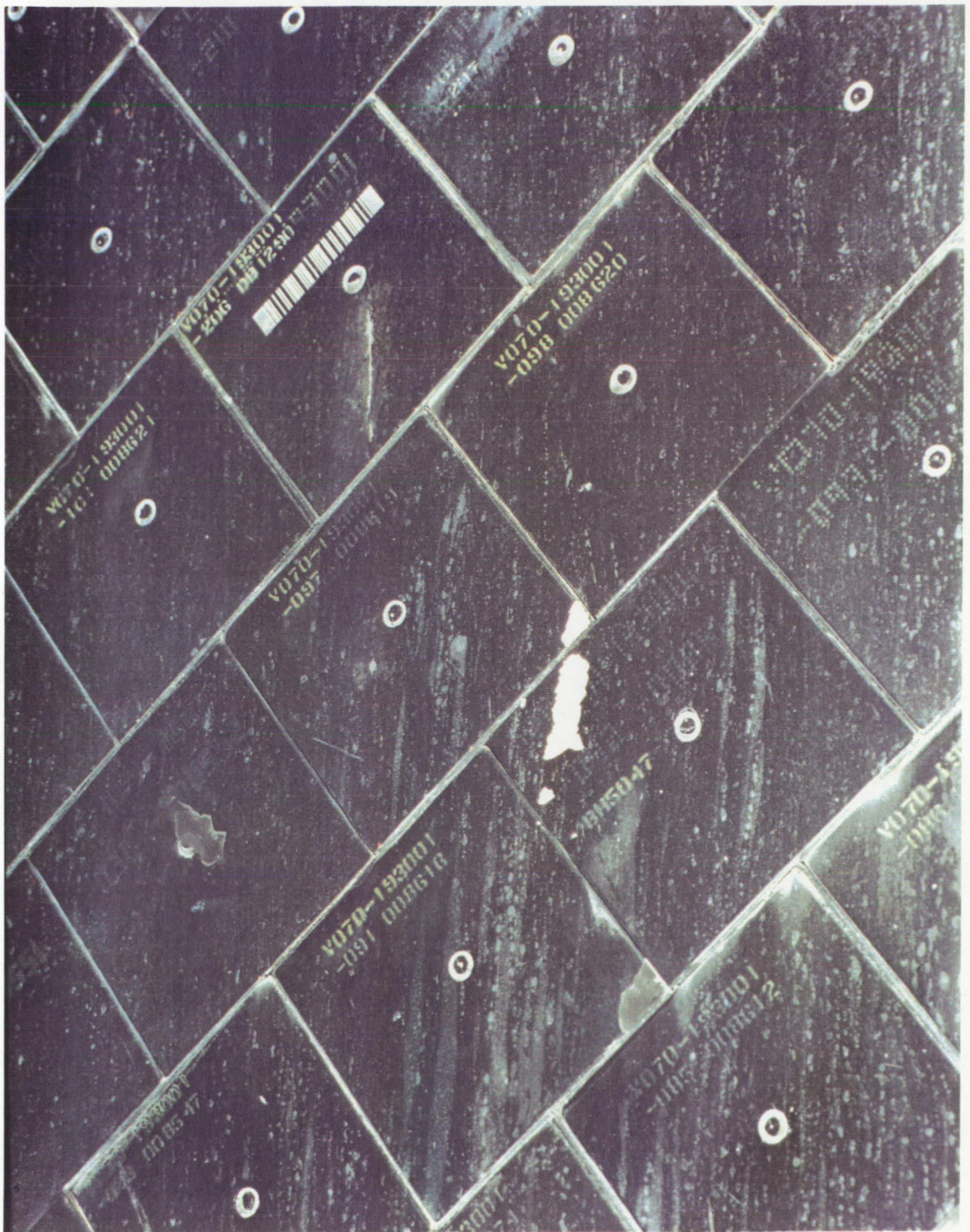
Typical debris impact damage to lower surface tiles
