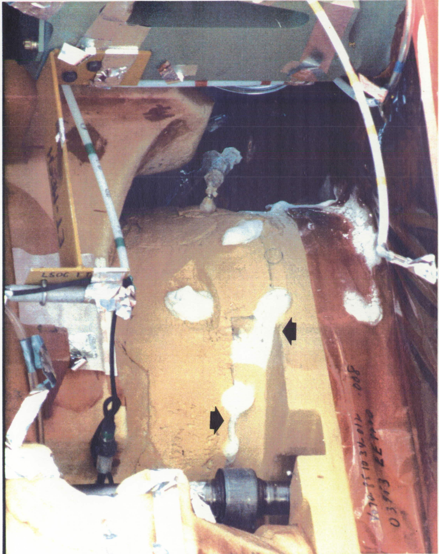
Due to the changing test configurations, numerous TPS cracks and isochem bondline thermal shorts were revealed by the appearance of ice/frost formations.
