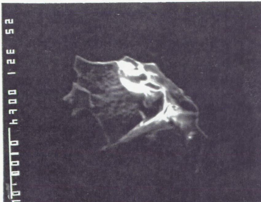
Figure 2. High magnification SEM photomicrograph of white particle from Figure 1. #3. 320x.
