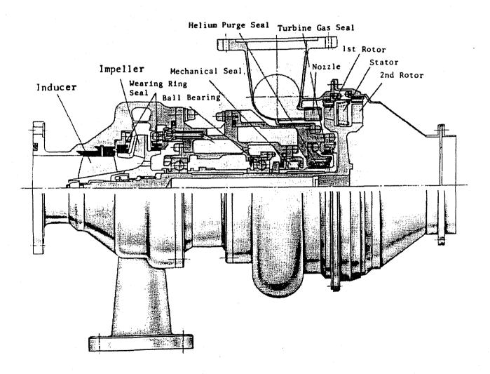
Figure 4.15. LE-5 Liquid Oxygen Turbopump
