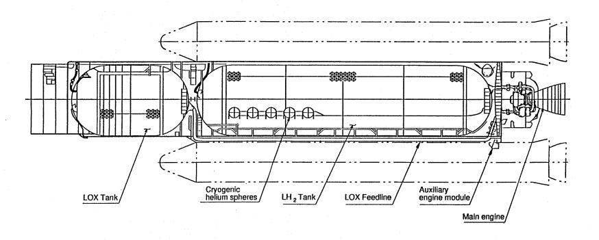
Figure 2.2 H-II Rocket First Stage Propulsion System
