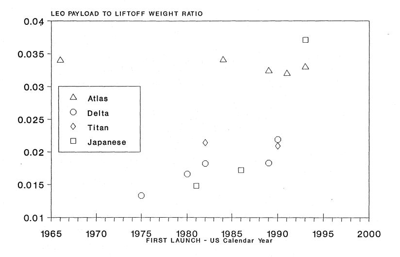
Figure 2.16 Vehicle Payload Efficiency Improvements
