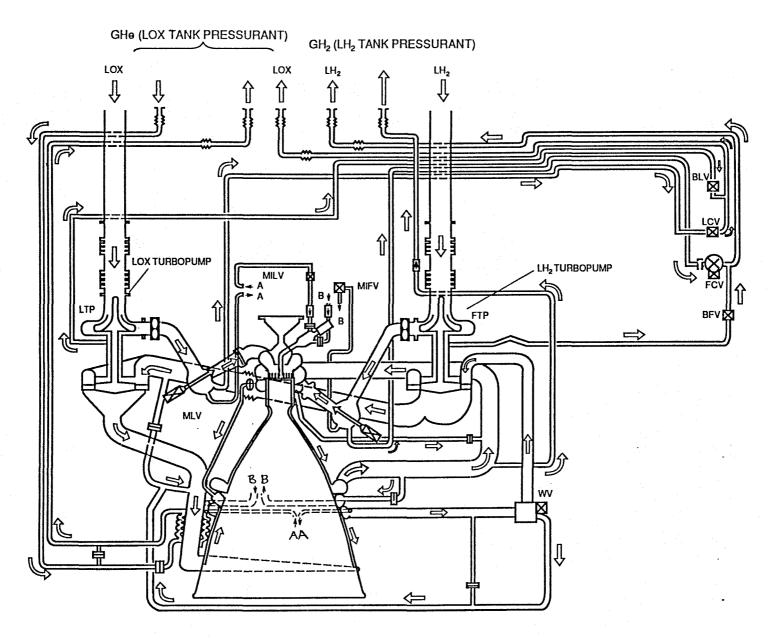
Figure 2.8 System Diagram of LE-5A Rocket Engine
