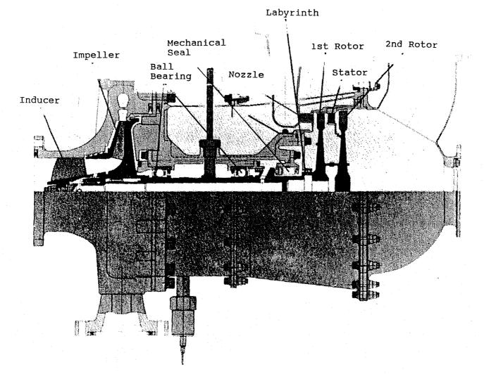
Figure 4.12. LE-5 Liquid Hydrogen Turbopump
