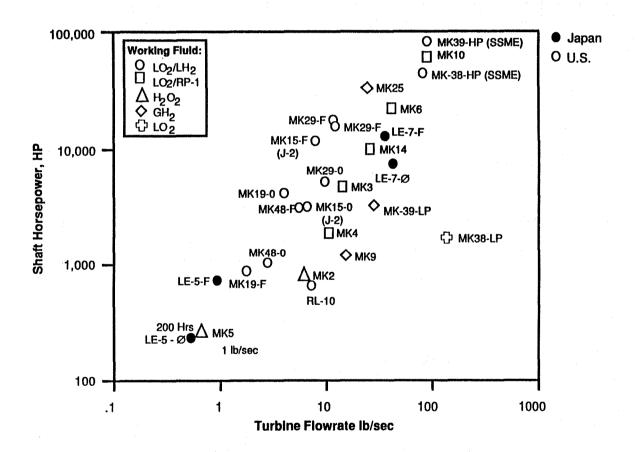
Figure 4.9. U.S. & Japanese Rocket Engine Turbines
