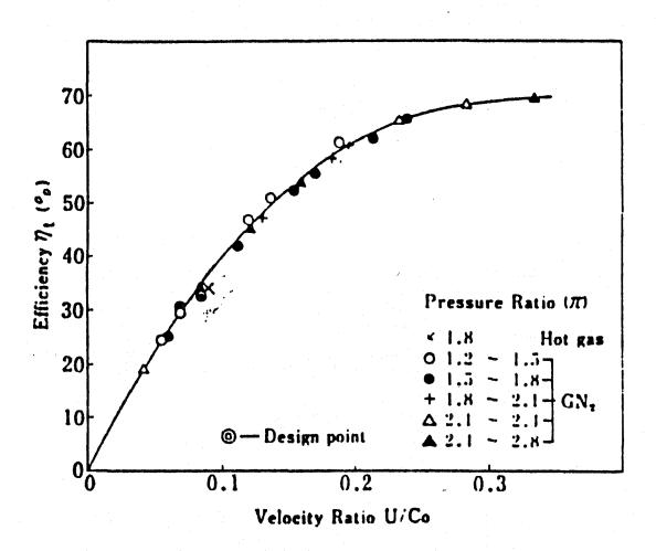
Figure 4.17. LE-5 LOX Turbopump Turbine Efficiency
