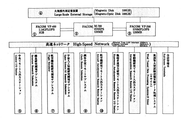
Figure 5.18. Numerical Simulator System at NAL
