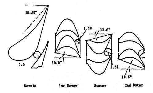
Figure 4.13. LE-5 Blade Profiles of LH<sub>2</sub> Turbopump Turbine
