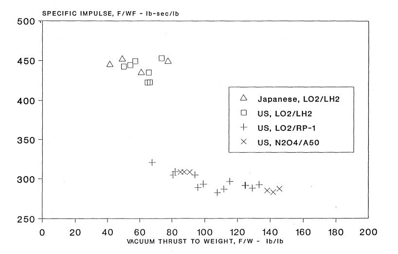
Figure 2.13 Rocket Engine Performance
