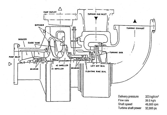
Figure 4.21. LE-7 Fuel Turbopump
