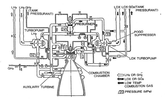
Figure 4.18. LE-7 Engine Schematic
