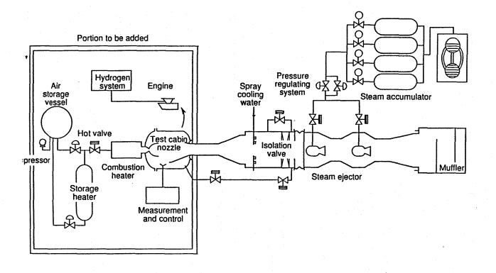
Figure 5.14. General Concept of the Scramjet Engine Test Facility
