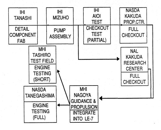
Figure 3.10. LE-7 Turbopump Assembly Flow
