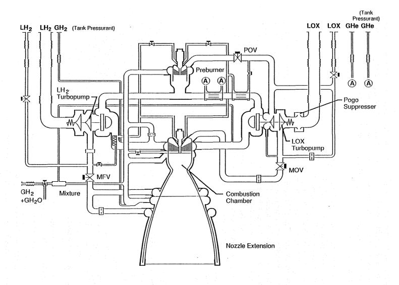
Figure 2.9 System Diagram of LE-7 Rocket Engine
