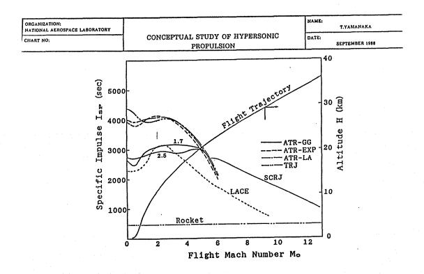
Figure 5.8. Comparison of Isp on the Flight Trajectory
