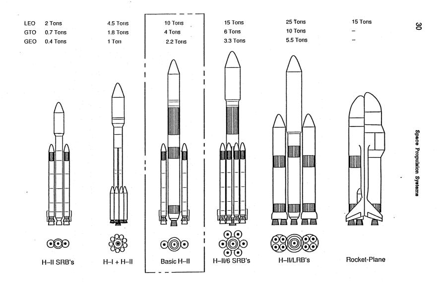
Figure 2.6 Concepts of H-II Derived Vehicles
