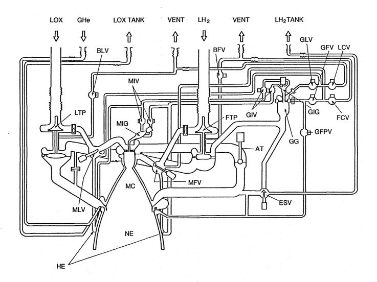
Figure 2.7 System Diagram of LE-5 Rocket Engine
