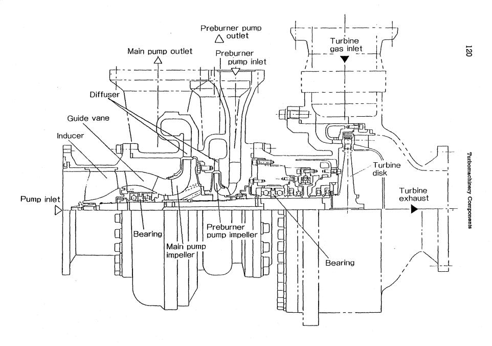
Figure 4.24. LE-7 LOX Turbopump
