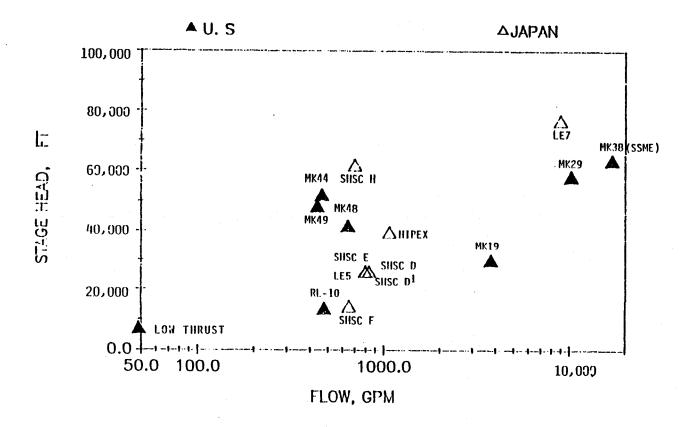
Figure 4.3. U.S. & Japanese LH<sub>2</sub> Centrifugal Pumps Stage Head vs. Flow
