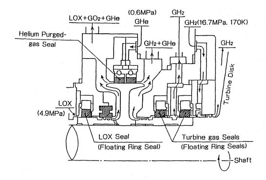
Figure 4.32. Japanese LE-7 LOX Turbopump Shaft seals
