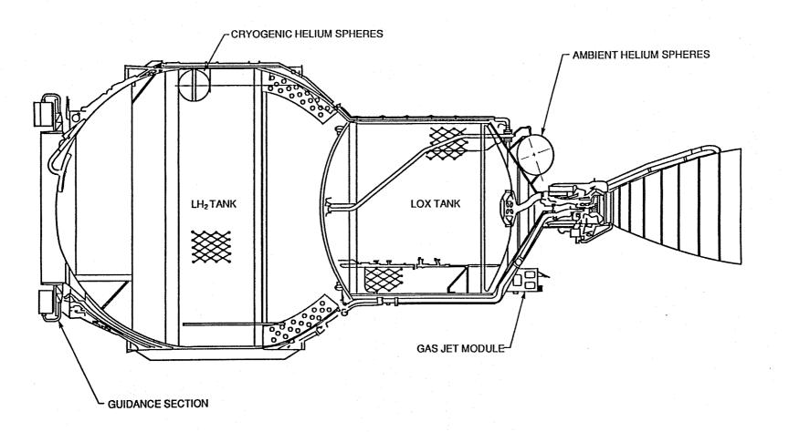
Figure 2.3 H-II Rocket Second Stage Propulsion System
