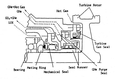
Figure 4.31. Japanese LE-5 LOX Turbopump Shaft Seals
