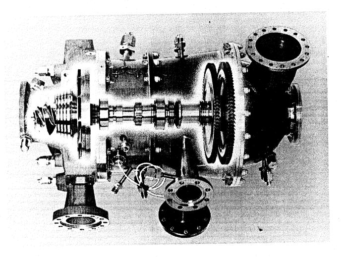
Figure 3.5. LE-5 Hydrogen Pump (Photo Courtesy IHI)
