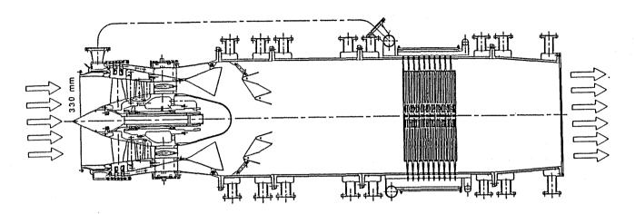
Figure 4.29. Configuration of ATREX-500 Engine
