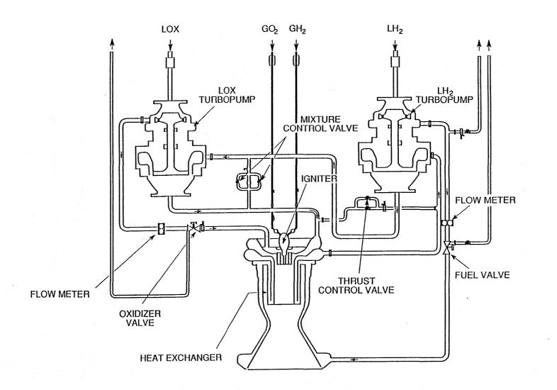
Figure 2.10 System Diagram of HIPEX-X01 Rocket Engine
