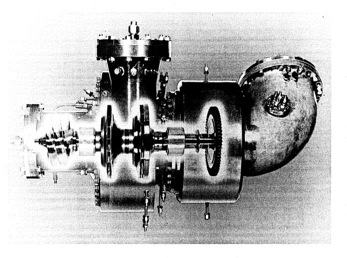
Figure 3.2. LE-7 Hydrogen Pump (Photo Courtesy IHI)
