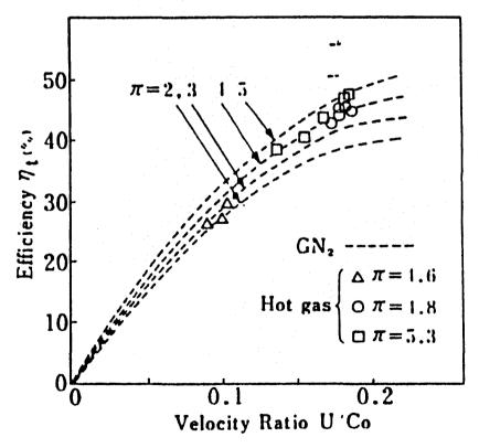
Figure 4.14. LE-5 LH<sub>2</sub> Turbopump Turbine Efficiency
