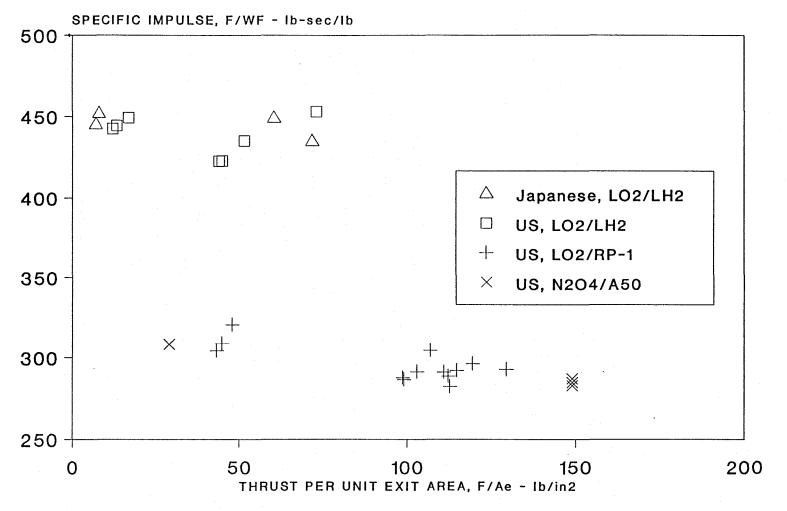
Figure 2.12 Engine Specific Impulse Comparison
