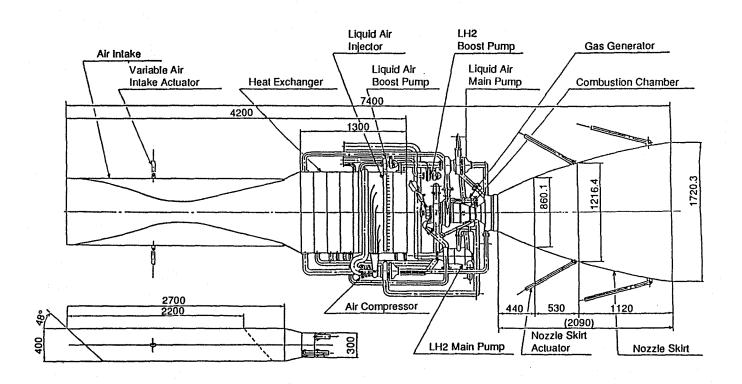
Figure 2.14 Experimental LACE Engine Based upon LE-5
