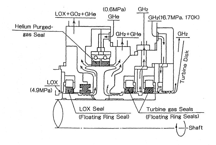
Figure 4.25. Shaft Seal System of LOX Turbopump
