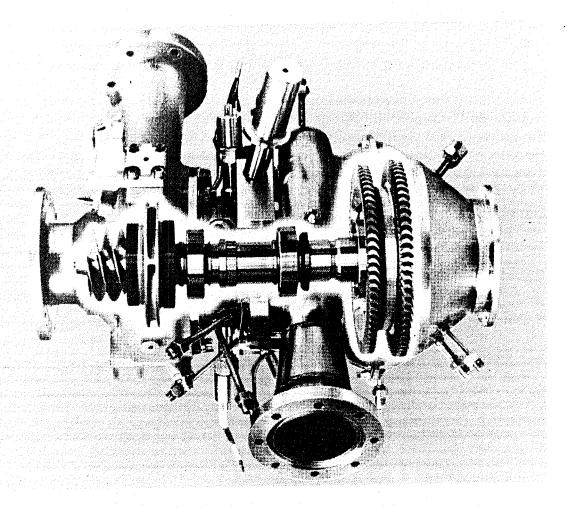
Figure 3.6. LE-5 Oxidizer Pump (Photo Courtesy NAL)
