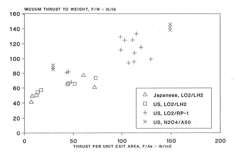
Figure 2.11 Engine Thrust to Weight Comparison
