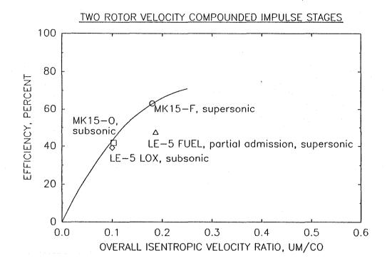
Figure 4.11. JTEC Turbine Comparisons
