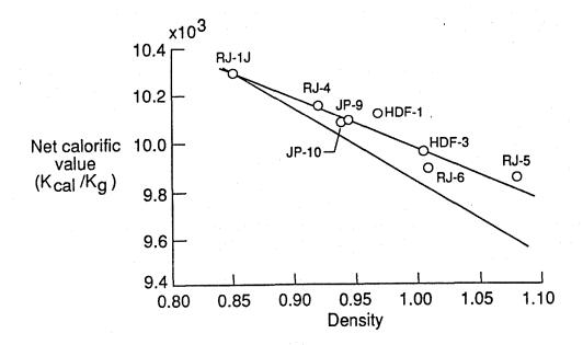
Figure 5.15. Net Calorific Value and Density
