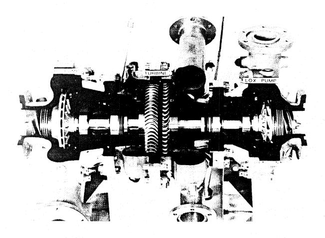
Figure 3.4. Early  $\rm H_2/\rm 0_2$  Engine Turbopump for 7 to 10 Ton Class Engines (Photo Courtesy IHI)
