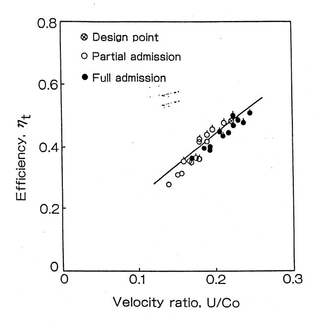
Figure 4.26. Overall Performance of Turbine
