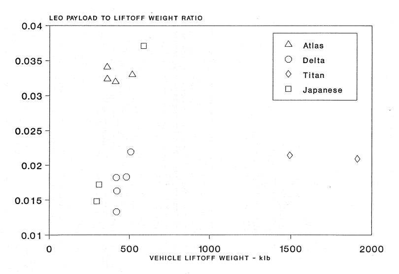
Figure 2.1 Vehicle Payload Efficiency
