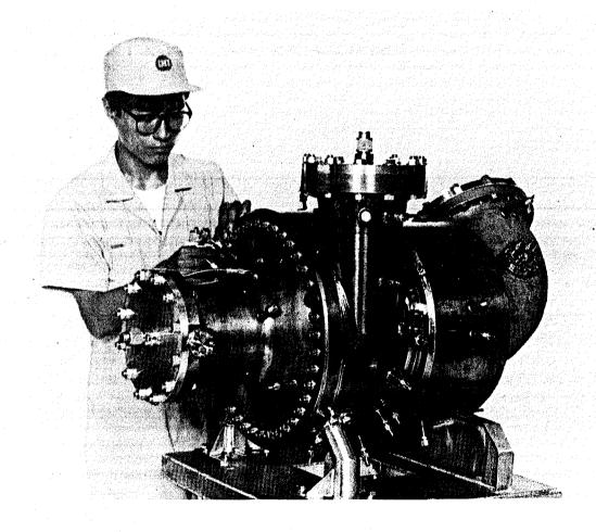
Figure 3.1. LE-7 Hydrogen Turbopump Assembly (Photo Courtesy IHI)
