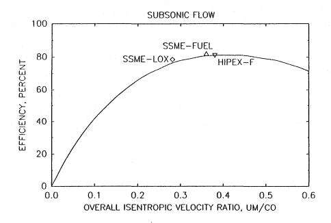
Figure 4.20. JTEC Turbine Comparisons Two Rotor Stages
