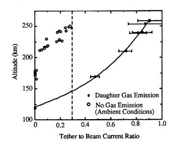
Figure 1 - Plot of tether to beam current ratio versus altitude with and without daughter gas emissions. The ratio of daughter to total (daughter plus mother) current collection areas, 0.29, is identified by the dashed line.
