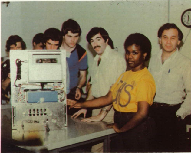
Camden and Woodrow Wilson High School students (Camden, N.J.) with GAS payload sponsored by RCA. The payload explored the colony behavior of ants in a weightless environment.
