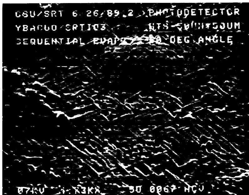
Figure 2. Higher magnification scanning electron micrograph of the bridge region of the sequentially evaporated detector.
