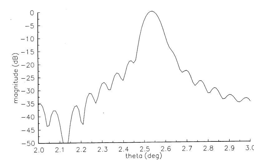
Figure 3.2-3. Radiation pattern of the Foldes Type 2 reflector antenna with correcting tertiary designed for the + 2.5° scan direction computed using MRAPCA. Feed pattern is  $\cos^q(\theta)$  with q selected to give a -10 dB tertiary edge illumination. Main reflector diameter is 933  $\lambda$ .
