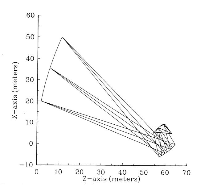
Figure 3.2-6. Gregorian Type 2A reflector antenna configuration designed to scan ± 2.5°. Main reflector diameter is 30 m, main reflector focal length is 56 m (F/D = 1.9). Elliptic subreflector diameter is 9.46 m. Shaped tertiary reflector diameter varies from 5.09 m to 6.56 m.
