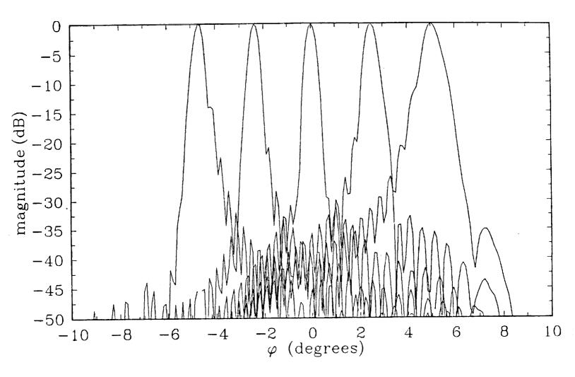
Figure 3.2-19. Radiation pattern of the Gregorian Type 2B reflector antenna with 6 m non-corrected tertiary designed for the 0° scan direction and rotated to obtain  $\pm$  5° scan computed using MRAPCA. Feed pattern is  $\cos^q(\theta)$  with q selected to give a -15 dB tertiary edge illumination. Main reflector diameter is 200  $\lambda$ .
