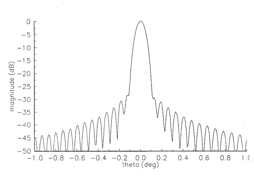
Figure 3.2-15. Radiation pattern of the Gregorian Type 2B reflector antenna with 6 m correcting tertiary designed for the +0° scan direction computed using MRAPCA. Feed pattern is  $\cos^q(\theta)$  with q selected to give a -15 dB tertiary edge illumination. Main reflector diameter is 1000  $\lambda$ .
