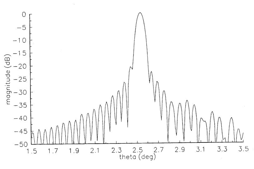
Figure 3.2-8 Radiation pattern of the Gregorian Type 2A reflector antenna with correcting tertiary designed for the + 2.5° scan direction computed using MRAPCA. Feed pattern is  $\cos^q(\theta)$  with q selected to give a -10 dB tertiary edge illumination. Main reflector diameter is 1000  $\lambda$ .
