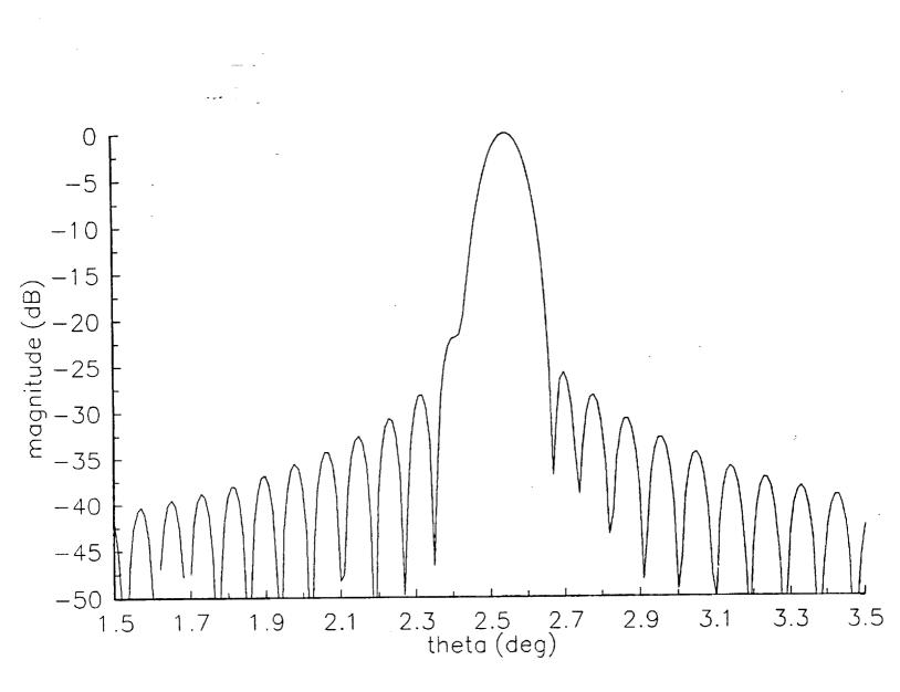
Figure 3.2-14. Radiation pattern of the Gregorian Type 2B reflector antenna with 6 m correcting tertiary designed for the +2.5° scan direction computed using MRAPCA. Feed pattern is  $\cos^q(\theta)$  with q selected to give a -15 dB tertiary edge illumination. Main reflector diameter is 1000  $\lambda$ .
