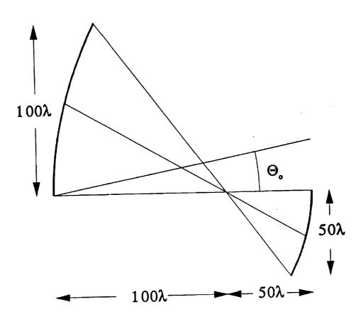
Figure 3.5-1. Geometry of a dual parabolic imaging reflector system.
