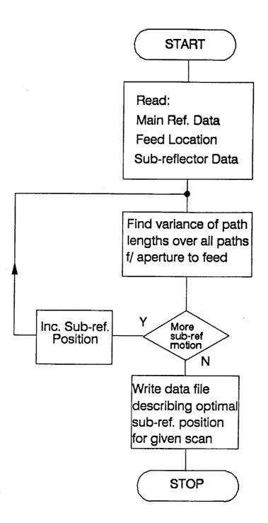
Figure 3.3-3 Two-dimensional statically shaped sub-reflector movement optimization sub-routine FITTER2D.FOR.
