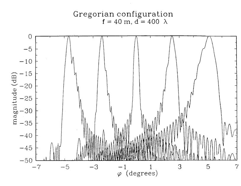
Figure 3.2-20. Radiation pattern of the Gregorian Type 2B reflector antenna with 6 m non-corrected tertiary designed for the 0° scan direction and rotated to obtain  $\pm$  5° scan computed using MRAPCA. Feed pattern is  $\cos^q(\theta)$  with q selected to give a -15 dB tertiary edge illumination. Main reflector diameter is 400  $\lambda$ . 5. An investigation into the possibility of using tertiary and feed translational movement to reduce the phase error of a fixed tertiary shape system.
