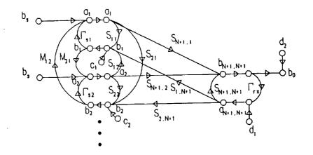
Figure 4-2. Generalized network model (signal flow graph) for an array and associated feed network. semiannu.al d:\wls 02/28/91
