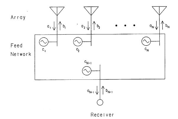
Figure 4-1. Model of array and feed network with noise sources.
