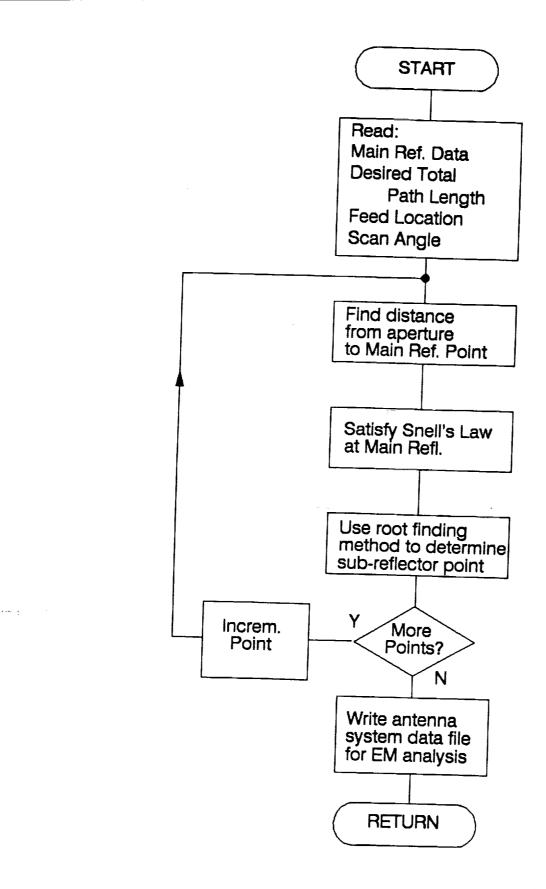
Figure 3.3-2 Two-dimensional dynamically reshaping subreflector generator subroutine RESHAP2D.FOR.
