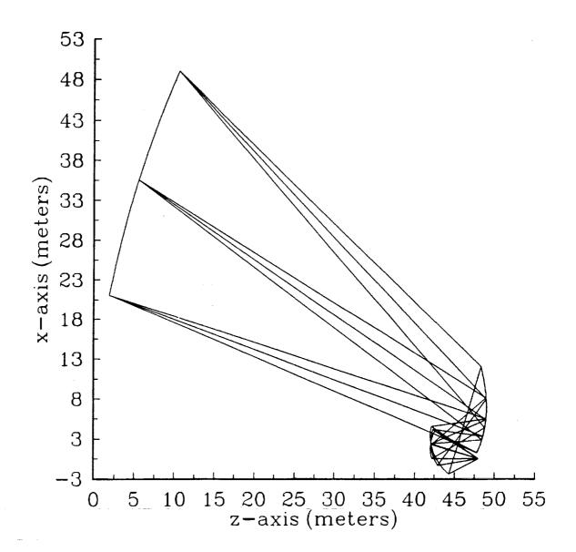
Figure 3.2-1. Foldes Type 2 (Cassegrain) reflector antenna configuration designed to scan ± 2.5°. Main reflector diameter is 28 m, main reflector focal length is 56 m (F/D=2). Elliptic subreflector diameter is 10.5 m. Shaped tertiary reflector diameter varies from 3.5 m to 6.7 m.
