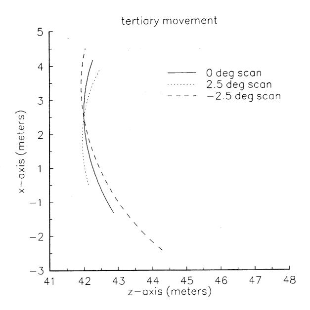
Figure 3.2-2. Tertiary reflector positions, sizes, and shapes for the Foldes Type 2 reflector (see Fig. 3.2-1) for the scan angles of +2.5°, 0°, and -2.5°.
