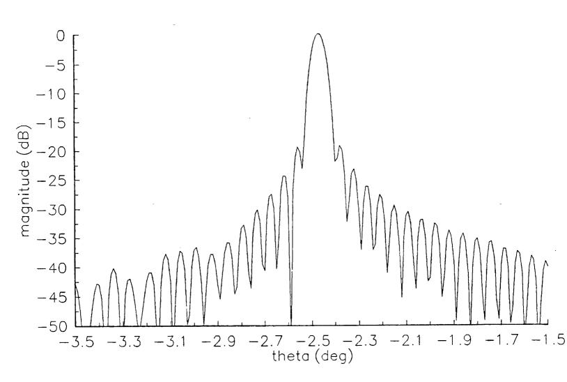
Figure 3.2-10. Radiation pattern of the Gregorian Type 2A reflector antenna with correcting tertiary designed for the -2.5° scan direction computed using MRAPCA. Feed pattern is  $\cos^q(\theta)$  with q selected to give a -10 dB tertiary edge illumination. Main reflector diameter is 1000  $\lambda$ .
