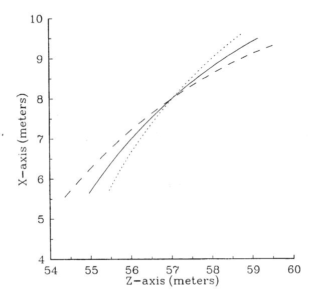
Figure 3.2-7. Tertiary reflector positions, sizes, and shapes for Gregorian Type 2A reflector system (see Fig. 3.2-6) for the scan angles of +2.5°, 0°, and -2.5°.
