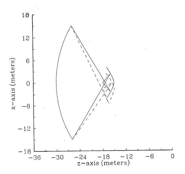
Figure 3.4-2. Scanning scenario for an "extended aperture efficiency spherical reflector antenna". An oversized subreflector and relative motion between the feed and subreflector allow for ±5° of scan with no spillover and no loss in aperture efficiency. Solid lines represents edge rays for 0° scan direction, perforated lines represents edge rays for +5° scan direction.
