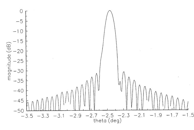
Figure 3.2-16. Radiation pattern of the Gregorian Type 2B reflector antenna with 6 m correcting tertiary designed for the -2.5° scan direction computed using MRAPCA. Feed pattern is  $\cos^q(\theta)$  with q selected to give a -15 dB tertiary edge illumination. Main reflector diameter is 1000  $\lambda$ .
