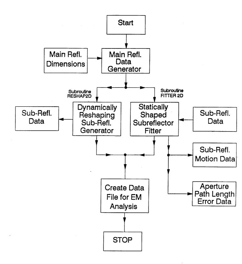
Figure 3.3-1 Subreflector Scan Movement Optimization Code - 2D (SSMOC) Data Flow Chart.
