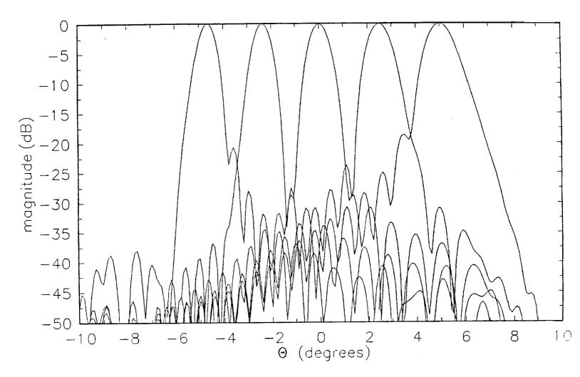
Figure 3.2-18. Radiation pattern of the Gregorian Type 2B reflector antenna with 6 m non-corrected tertiary designed for the 0° scan direction and rotated to obtain  $\pm$  5° scan computed using MRAPCA. Feed pattern is  $\cos^q(\theta)$  with q selected to give a -15 dB tertiary edge illumination. Main reflector diameter is 100  $\lambda$ .
