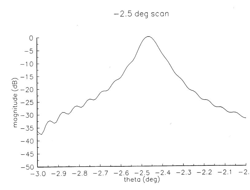
Figure 3.2-5. Radiation pattern of the Foldes Type 2 reflector antenna with correcting tertiary designed for the -2.5° scan direction computed using MRAPCA. Feed pattern is  $\cos^q(\theta)$  with q selected to give a -10 dB tertiary edge illumination. Main reflector diameter is 933  $\lambda$
