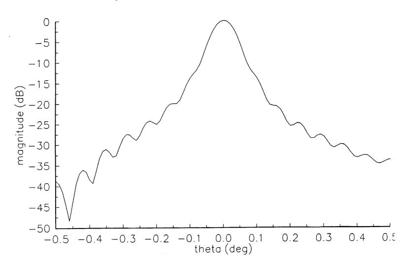
Figure 3.2-4. Radiation pattern of the Foldes Type 2 reflector antenna with correcting tertiary designed for the 0° scan direction computed using MRAPCA. Feed pattern is  $\cos^q(\theta)$  with q selected to give a -10 dB tertiary edge illumination. Main reflector diameter is 933  $\lambda$
