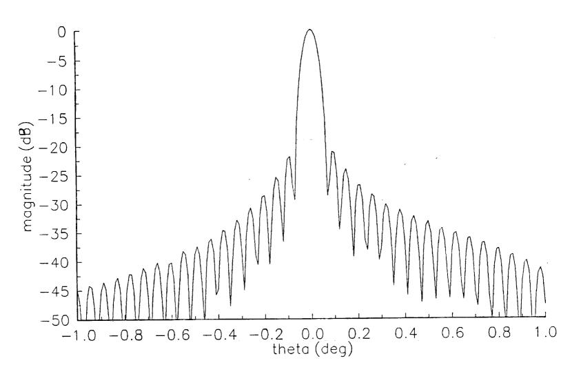
Figure 3.2-9 Radiation pattern os the Gregorian type 2(a) reflector antenna with correcting tertiary designed for the 0° scan direction computed using MRAPCA. Feed pattern is  $\cos^q(\theta)$  with q selected to give a -10 dB tertiary edge illumination. Main reflector diameter is 1000  $\lambda$
