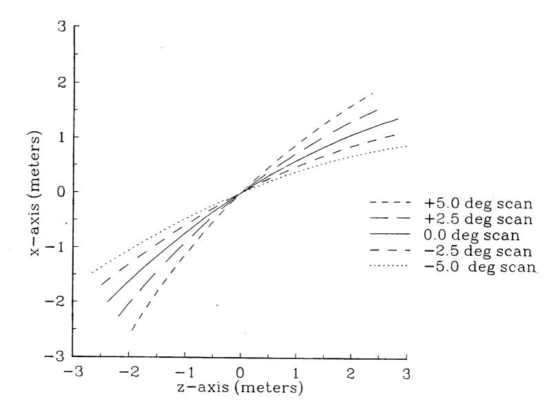
Figure 3.2-12. Tertiary reflector positions and shapes for the Gregorian Type 2B reflector system (see Fig. 3.2-11) for scan angles of +5°, +2.5°, 0°, -2.5°, and -5°. All tertiary diameters reduced to approximately 6 m.
