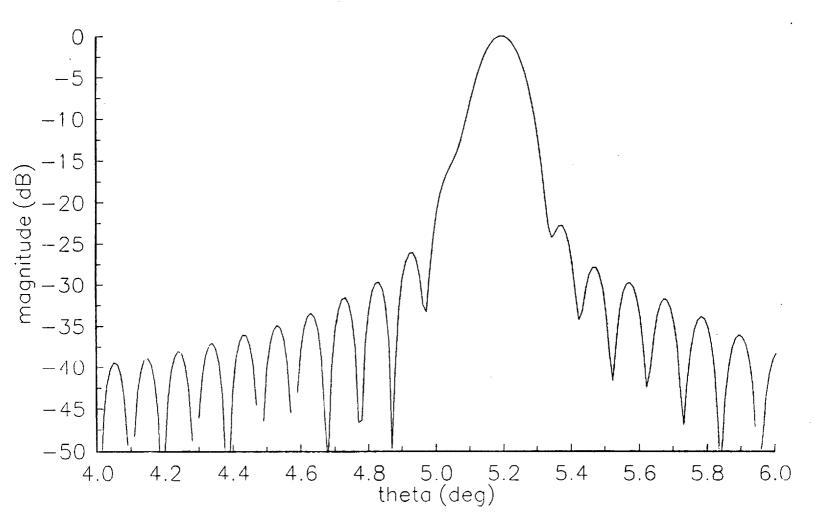
Figure 3.2-13. Radiation pattern of the Gregorian Type 2b reflector antenna with 5 m correcting tertiary designed for the +5 scan direction computed using MRAPCA. Feed pattern is  $\cos^q(\theta)$  with q selected to give a -15 dB tertiary edge illumination. Main reflector diameter is 1000  $\lambda$ .
