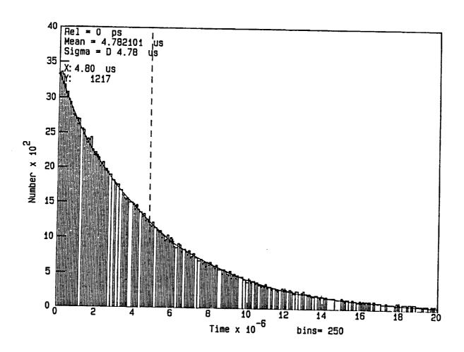
Figure 22. Histogram of the interarrival times under 1 pW received optical power. The solid curve corresponds to the exponential distribution with the same mean (i.e.  $3308exp\left[-t/4.78\times10^{-6}\right]$ ). The sample size was  $2\times10^{5}$ .
