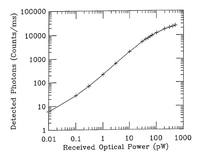
Figure 24. Average number of detected counts of the experimental nonbreak-down APD photon counter versus received optical power in pW.
