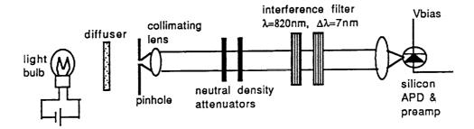
Figure 11. Optical Setup of the Experiment.
