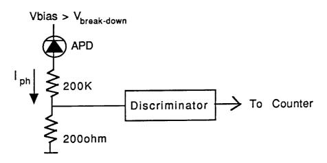
Figuire 3. Avalanche break-down APD photon counter.
