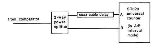
Figure 21. Apparatus used for measuring interarrival times.
