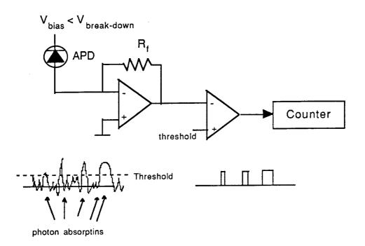
Figure 6. Circuit diagram of nonbreak-down APD photon counter.
