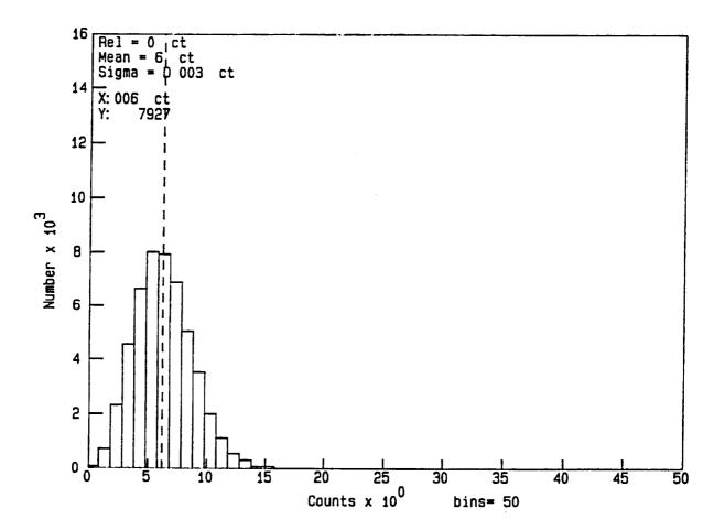
Figure 19. Histogram of the number of the total measured dark counts over a 1 ms counting interval. The sample size was  $5\times10^4$ .
