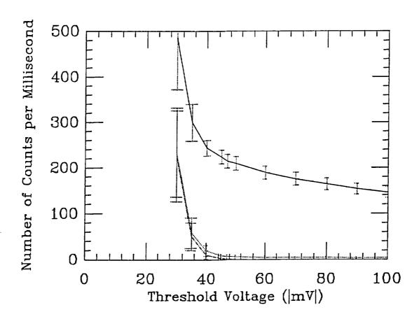
Figure 17. Average number and standard deviation (solid curve) of the detected counts in 1 ms under 1 pW received optical power as a function of the threshold voltage applied at the comparator. The dot-dashed and the dotted curves represent the circuit thermal noise counts (APG gain G=0) and the total dark counts (G~1000), respectively.
