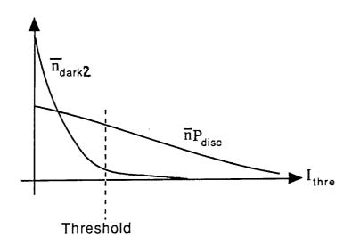
Figuire 10. Average numbers of detected photons and dark counts as a function of the threshold.
