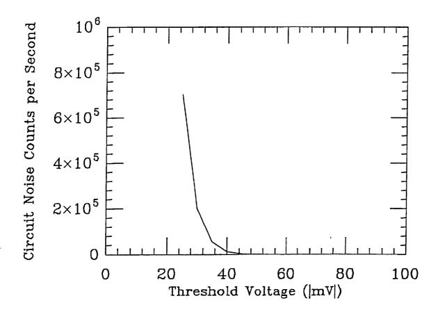
Figure 15. Circuit thermal noise counts versus threshold voltage applied at the comparator.
