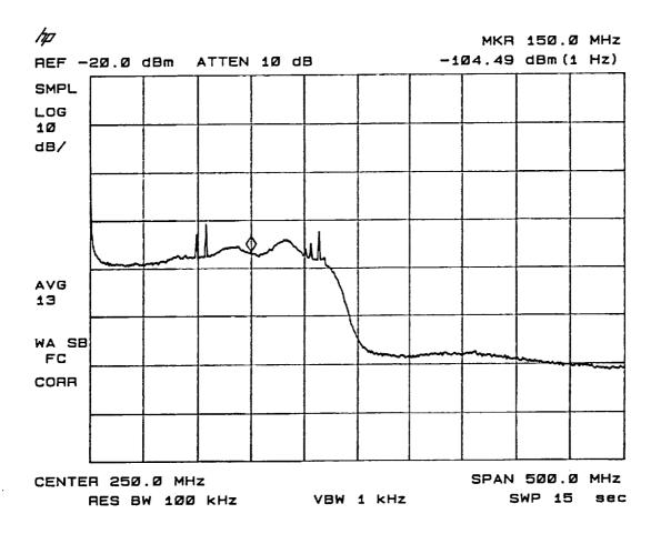
Figure 14. Power spectrum of the total circuit thermal noise measured at the input of the comparator.
