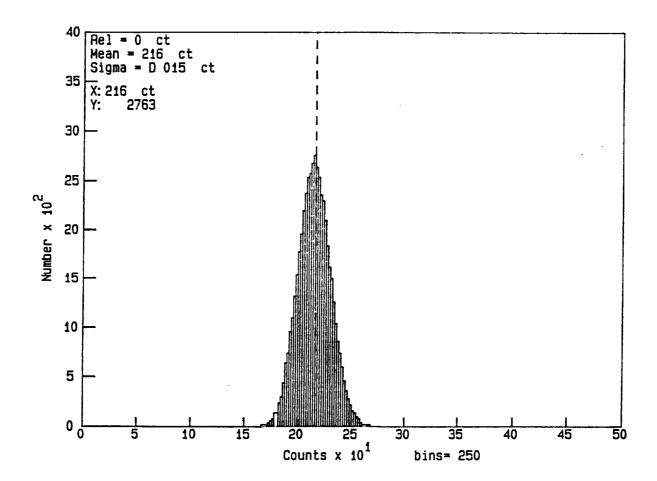
Figure 20. Histogram of the number of the detected counts under 1 pW received optical power over a 1 ms counting interval. The sample size was  $5\times10^4$ .
