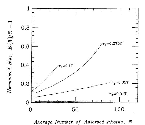
Figure 4. Normalized bias of the ML estimator,  $E\{\hat{n}\}$ , as a function of the average number of absorbed photons,  $\overline{n}$ .
