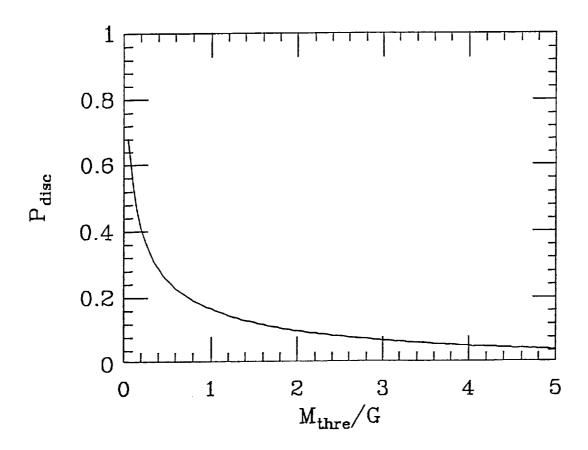
Figure 9. Probability of discrimination,  $P_{\it disc}$ , of a nonbreak-down APD photon counter versus the equivalent threshold gain,  $M_{\it thre}$ .
