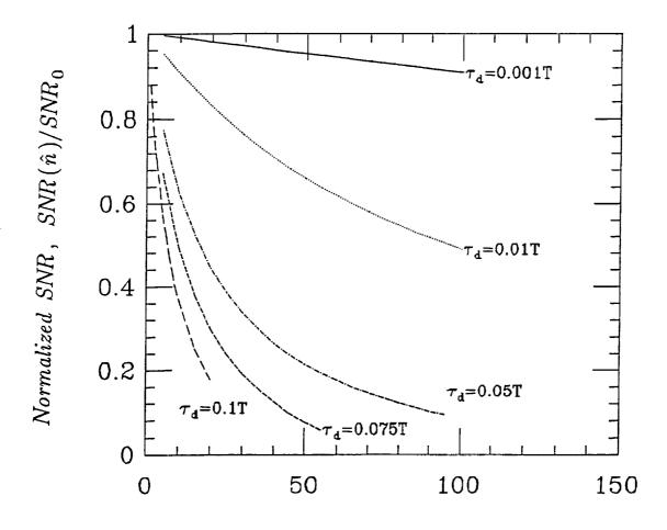
Figure 5. Normalized SNR of the ML estimator  $SNR(\hat{n})$  as a function of the average number of absorbed photons,  $\bar{n}$ . for a given dead time of  $\tau_d$  and a counting interval of T seconds.
