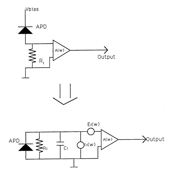
Figure 1. High input impedance APD preamplifier.
