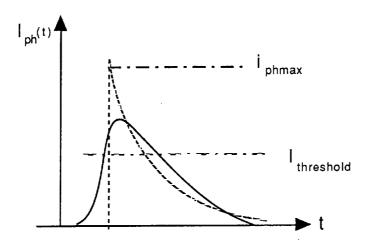
Figure 7. Photocurrent pulse shape. The dashed line represents the ideal exponential pulseshape and the solid line represents a more realistic pulseshape.
