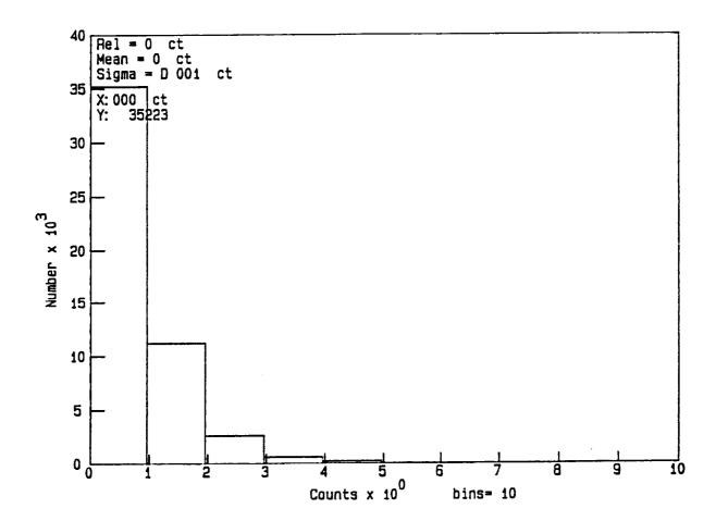
Figure 18. Histogram of circuit thermal noise noise counts over a 1 ms counting interval. The sample size was  $5\times10^4$ .
