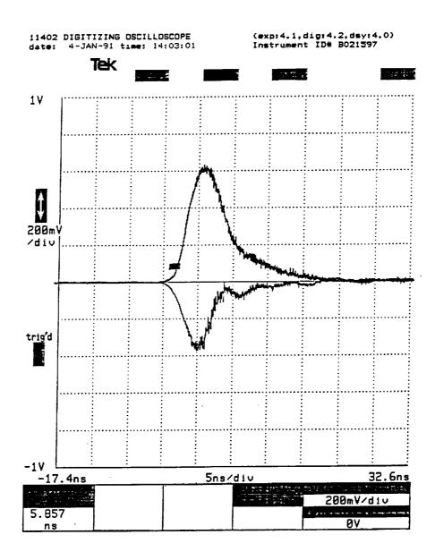
Figure 16. Average waveforms of input pulses (negative going) and output pulses (positive going) of the comparator.
