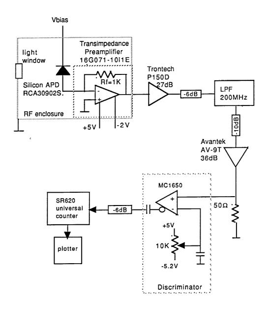
Figure 12. Non break-down APD photon counter circuit.
