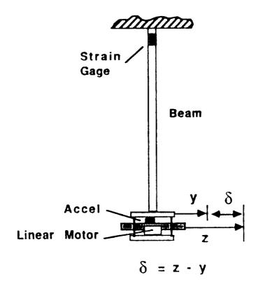
A block diagram of the feedback loops demonstrated on the test beam is shown here. For all tests, reaction mass relative position feedback was used to ensure the reaction mass remained centered. For damping augmentation of the beam, strain gage, beam acceleration, or reaction mass acceleration was used.
