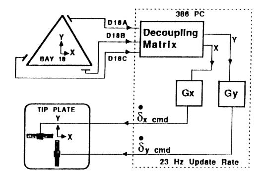
The Mini-Mast was excited for 9.8 seconds at the 1st bending mode frequency (.85 Hz) with both reaction mass actuators, followed by the feedback control at 10 seconds. The structural damping was increased from the 4.5 % free decay damping to approximately 15 % with displacement feedback.
