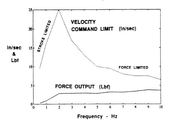
Using two actuators connected to the indexer causes the command update rate to decrease to approximately 106 Hertz. With the analog command input mode used and an accelerometer attached to the reaction mass, a dynamic signal analyzer was used to perform sine sweep tests over a frequency range of 0.5 to 6 Hz. The transfer function shown is actuator force output over velocity command input. This frequency response shows the expected results using a velocity command actuator.
