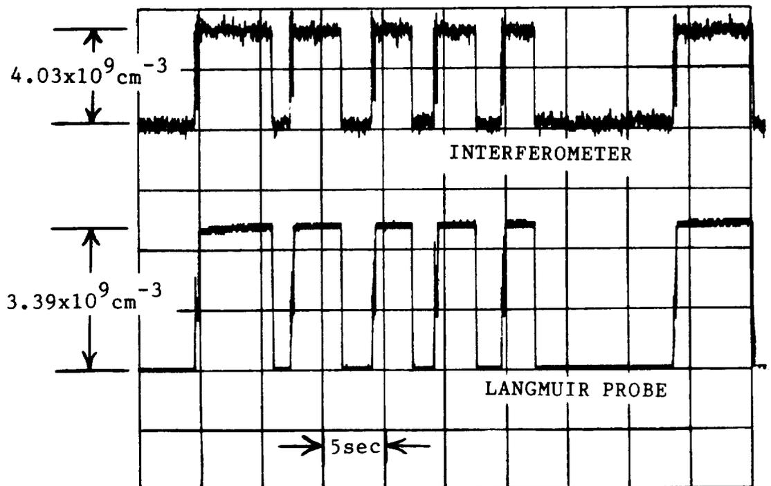
Figure 2. Calibration of Langmuir probe with microwave interferometer.
