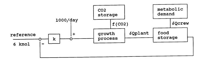
Figure 1. A block diagram of the planting control system.
