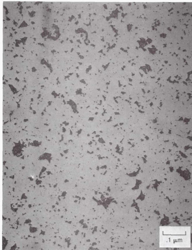
Figure 1.—Optical photomicrograph of Ag/Ti film on polished ( \approx 0.1 \mu\text{m} rms surface finish) \text{Al}_2\text{O}_3 disk specimen. Magnification is 100x. Black spots are pores due to pits and nonuniformities of \text{Al}_2\text{O}_3 substrate surface.
