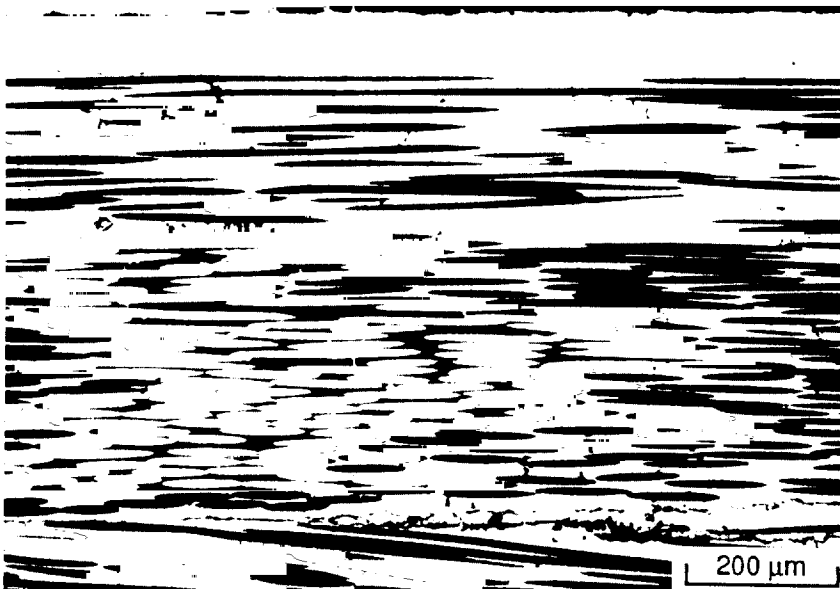
Figure 7.2-2 Longitudinal Photomicrograph of a Diffusion Bonded P100/6061 Al Tube Showing Transverse Microcracks in the Interfiber Matrix Region Observed in Both Diffusion Bonded and Pultruded Tubes (100X)
