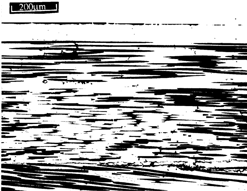
Figure 7.1-2 Longitudinal Micrograph of Diffusion Bonded 2-ply P100/6061 Al Panel Showing A Few Microcracks in the Interfiber Matrix Region
