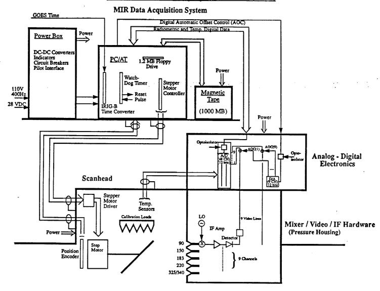
Figure 2. MIR block diagram, illustrating components in the scanhead and data acquisition system.
