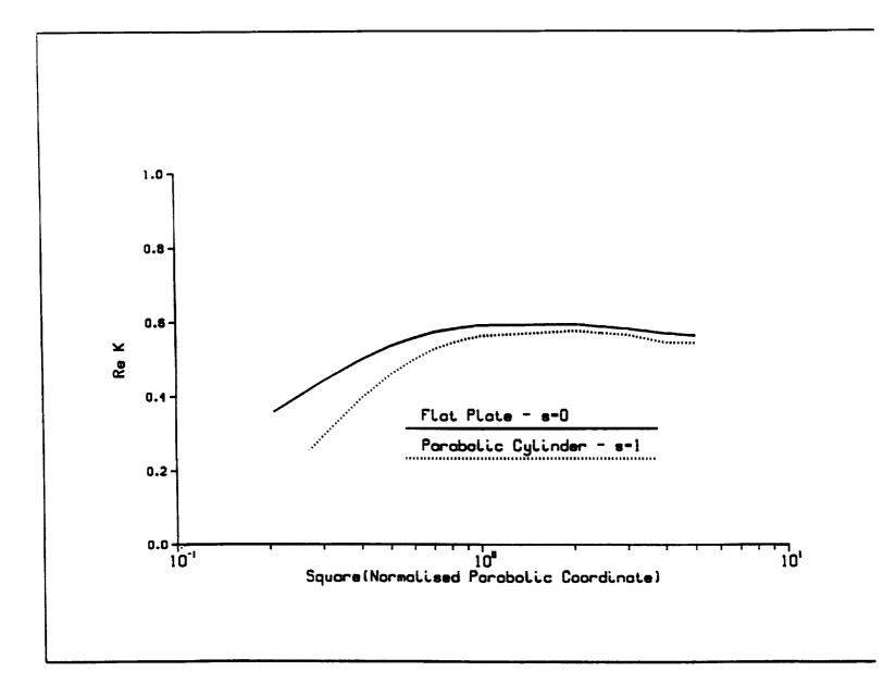
FIGURE 2. Variation of the real part of the TS wavenumber (multiplied by  $\epsilon$ ) as a function of the downstream distance (Re( $\kappa$ ) vs.  $\tilde{\xi}_1^2 = (\xi_1/U_0')^2$ ) for  $\epsilon \equiv (\omega\nu/U_{\infty}^2)^{-\frac{1}{6}} = 0.1$ . The flat plate result is compared to that for a parabolic surface with  $s \equiv \omega r_n/U_{\infty} = 1.0$ , where  $r_n$  is the nose radius.
