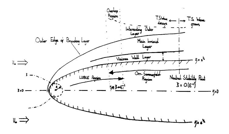
FIGURE 1. The asymptotic structure for the unsteady disturbances in the boundary layer of a parabolic cylinder.
