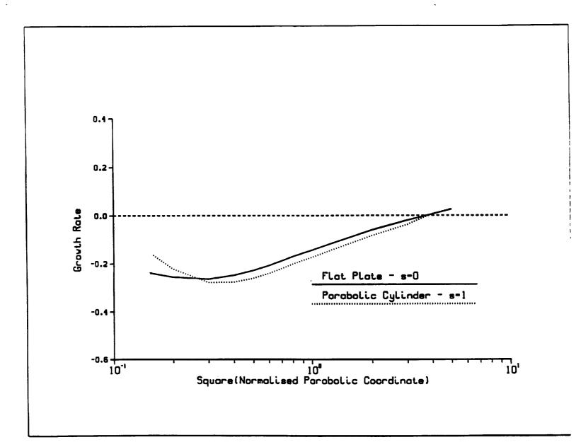
FIGURE 3. Variation of the growth rate of the TS wave (multiplied by  $\epsilon$ ) as a function of the downstream distance  $(-\text{Im}(\kappa) \text{ vs. } \tilde{\xi}_1^2 = (\xi_1/U_6')^2)$ . Flat plate results are compared with those for a parabolic cylinder with s = 1. The stabilising effect of the favourable pressure gradient can be seen, this effect decreasing with distance downstream as the body curvature approaches zero.
