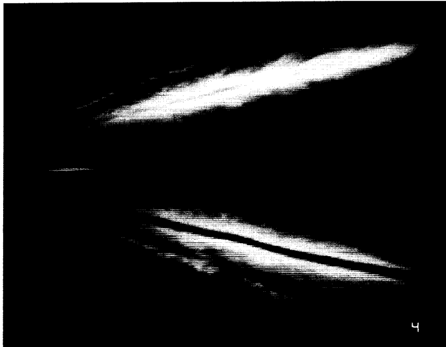
Figure A35. Longitudinal laser sheet cross section. Sweep = 70^\circ , Alpha = 30^\circ , U = 3.0 m/s.
