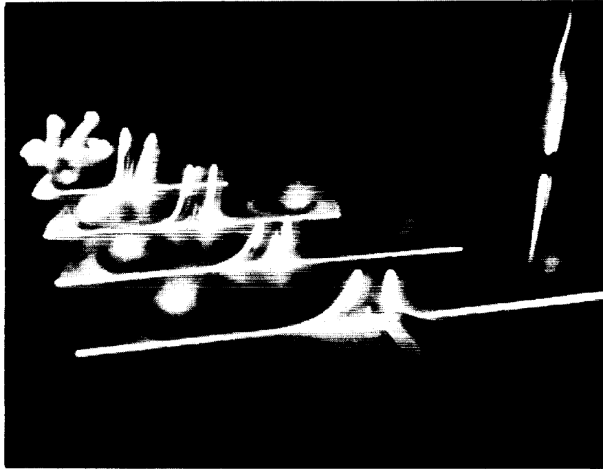
Figure A17. Lateral laser sheet cross sections. Sweep = 70^\circ , Alpha = 10^\circ , U = 3.0 m/s.
