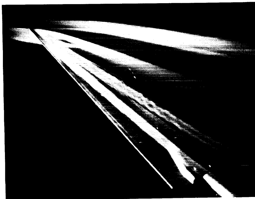
Figure A14. Smoke flow visualization with flood lamp illumination. Sweep = 85^\circ , Alpha = 20^\circ , U = 3.0 m/s.
