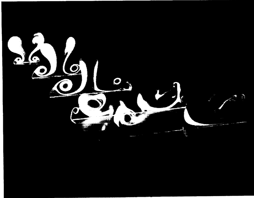
Figure A25. Lateral laser sheet cross sections. Sweep = 80^\circ , Alpha = 10^\circ , U = 3.0 m/s.
