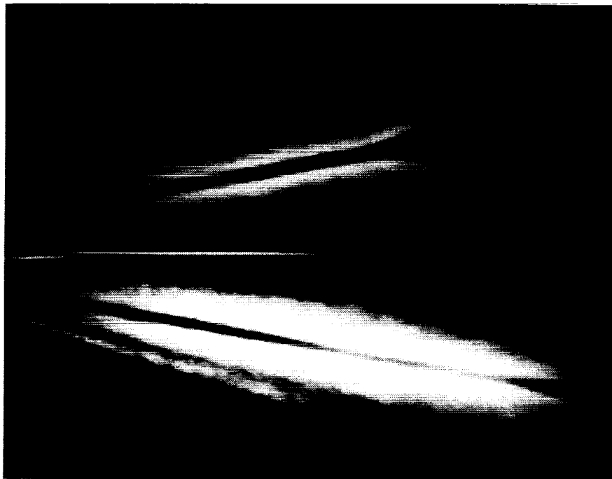
Figure A40. Longitudinal laser sheet cross section. Sweep = 75^\circ , Alpha = 40^\circ , U = 3.0 m/s.
