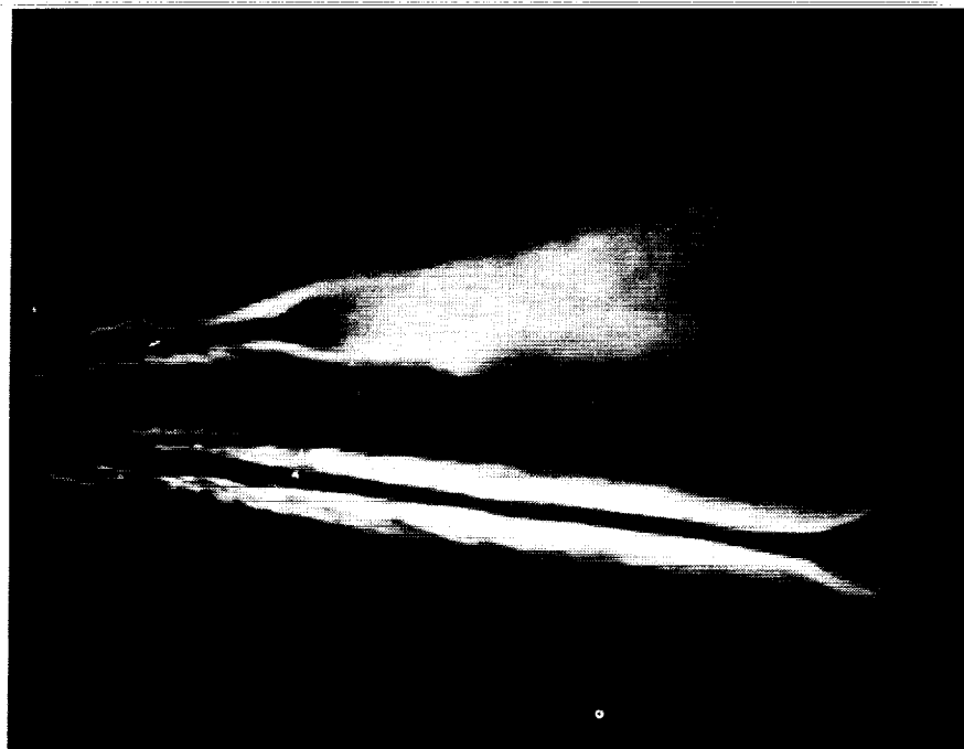
Figure A44. Longitudinal laser sheet cross section. Sweep = 80^\circ , Alpha = 40^\circ , U = 3.0 m/s.
