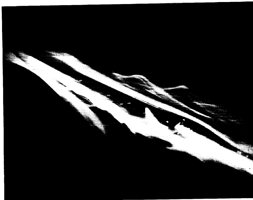
Figure A9. Smoke flow visualization with flood lamp illumination. Sweep = 80^\circ , Alpha = 10^\circ , U = 3.0 m/s.
