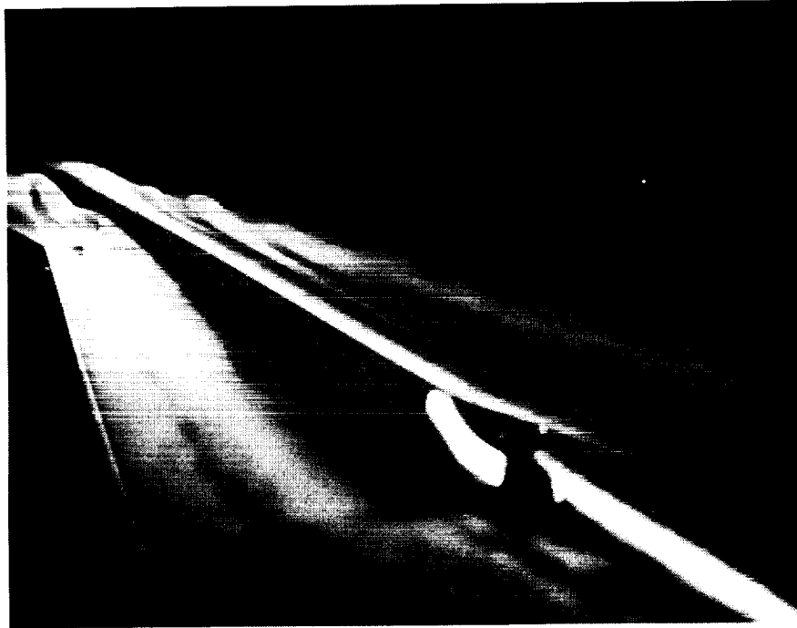
Figure A1. Smoke flow visualization with flood lamp illumination. Sweep = 70^\circ , Alpha = 10^\circ , U = 3.0 m/s.
