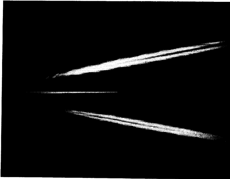
Figure A39. Longitudinal laser sheet cross section. Sweep = 75^\circ , Alpha = 30^\circ , U = 3.0 m/s.
