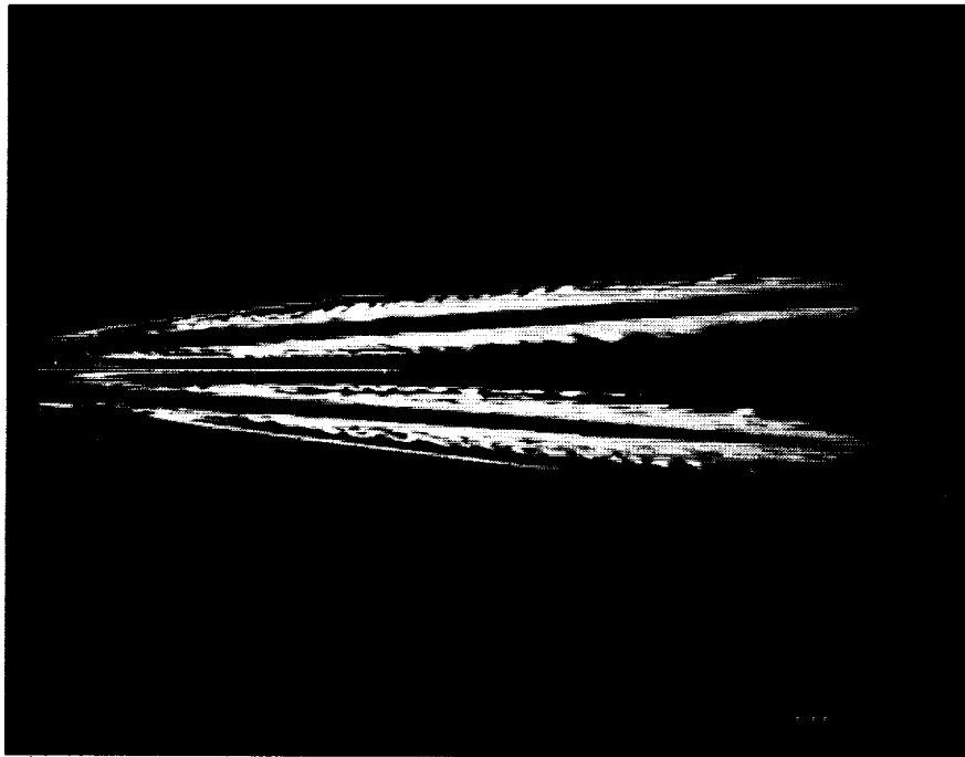
Figure A47. Longitudinal laser sheet cross section. Sweep = 85^\circ , Alpha = 30^\circ , U = 3.0 m/s.
