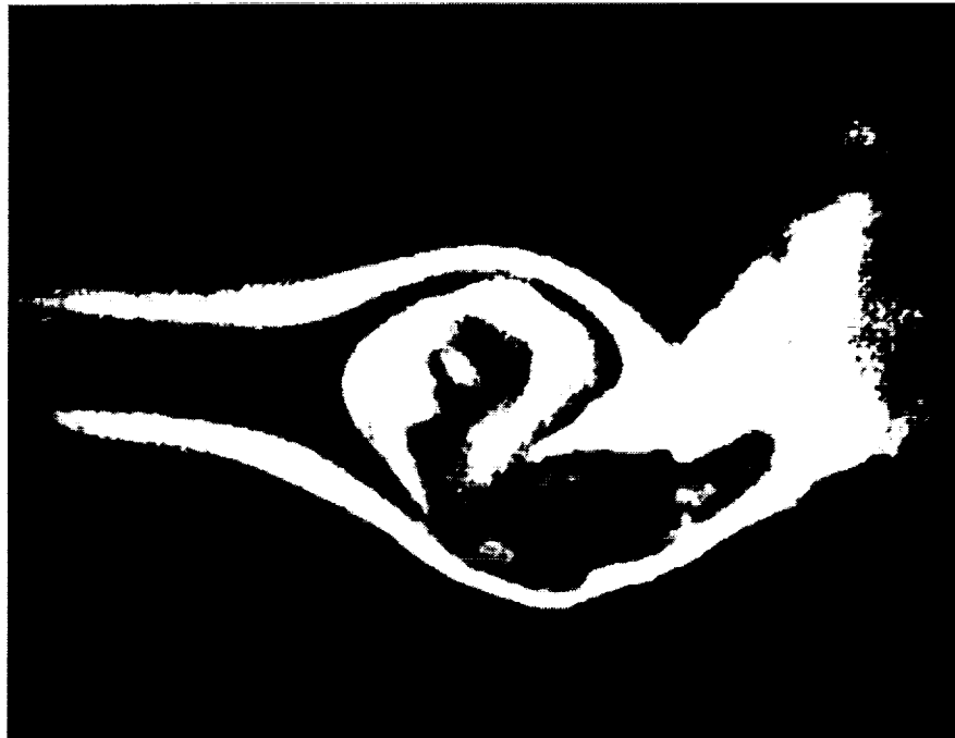
Figure 3.11 Asymmetric bubble type breakdown. Longitudinal cross section. Enlargement of 16mm movie frame.
