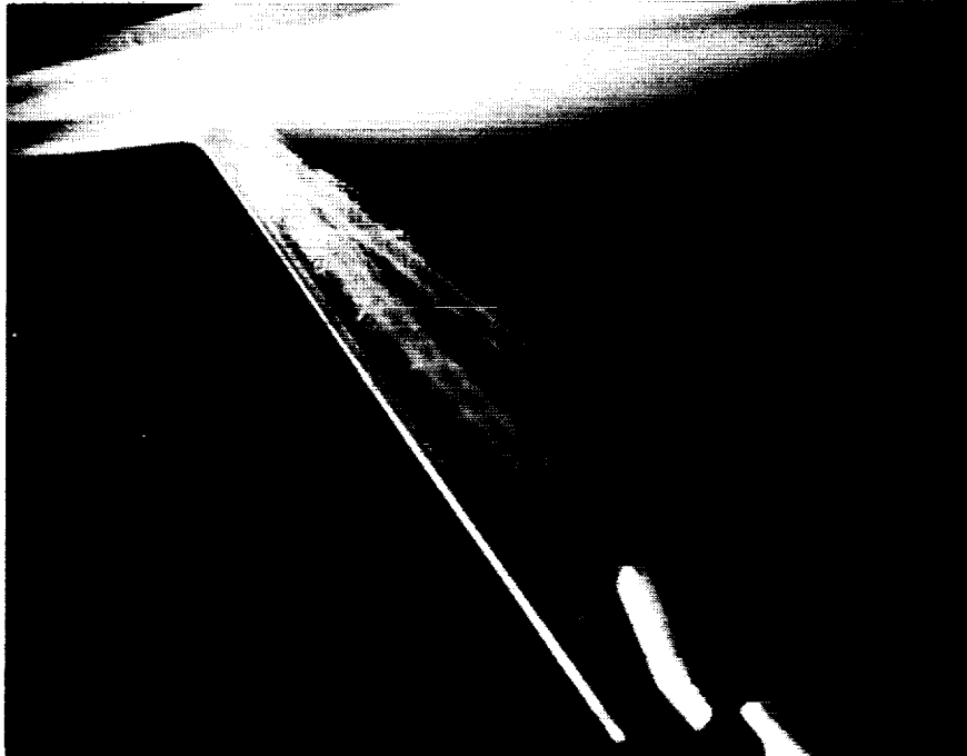
Figure A15. Smoke flow visualization with flood lamp illumination. Sweep = 85^\circ , Alpha = 30^\circ , U = 3.0 m/s.
