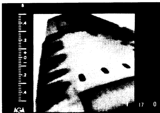
Fig. 7. The VFW-614 Advanced Technologies Testing Aircraft System. a) Schematic drawing; the laminar flow glove, marked gray, is outboard the engine pylon. 57 b) Close-up view of the wing area; notice the laminar glove and the IR cameras locations. 71 c) In-flight transition pattern induced by Tollmien-Schlichting waves and insect contamination (turbulent wedges). Courtesy A. Quast, DLR Braunschweig, reprinted with permission.
