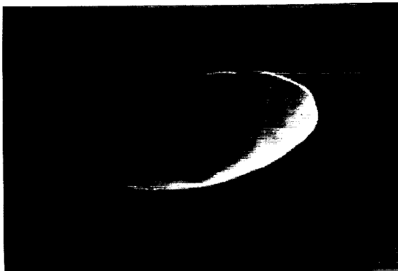
Figure 7 - Scanning Electron Photomicrograph of Plasma Ashed (to a fluence of 1.28 \times 10^{22} atoms/cm 2 ) and Tape Peeled Defects on 1300Å SiO x Coated Kapton with a Small Defect-Width-to-Coating Thickness Ratio.
