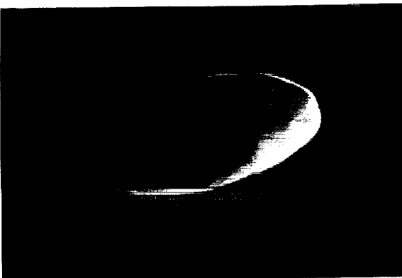
Figure 7 - Scanning Electron Photomicrograph of Plasma Ashed (to a fluence of 1.28 \times 10^{22} atoms/cm 2 ) and Tape Peeled Defects on 1300Å SiO x Coated Kapton with a Small Defect-Width-to-Coating Thickness Ratio.
