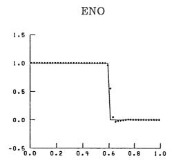
Fig. 4a. Numerical results at t = 0.3 using ENO scheme with discontinuous initial data and  $\mu = 1000$ .  $\Delta x = 0.02, \Delta t = 0.0075, -----:$  true solution,  $\cdots$ : computed solution
