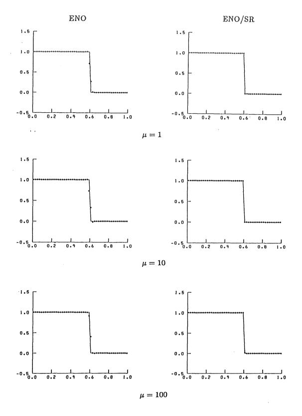
Fig. 3. Numerical results at t = 0.3 using ENO (first column) and ENO/SR (second column) schemes with discontinuous initial data for  $\mu = 1$  (first row),  $\mu = 10$  (second row), and  $\mu = 100$  (third row).  $\Delta x = 0.02$ ,  $\Delta t = 0.015$ , -----: true solution, ...: computed solution
