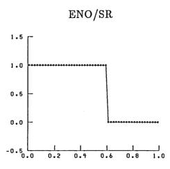
Fig. 4b. Numerical results at t = 0.3 using ENO/SR scheme with discontinuous initial data and  $\mu = 1000$ .  $\Delta x = 0.02, \Delta t = 0.0075, ----:$  true solution,  $\cdots$ : computed solution
