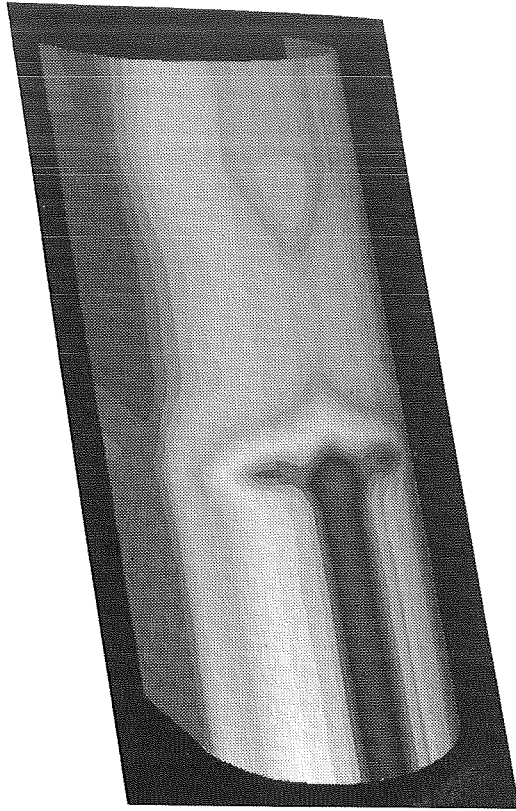
Figure 17: Surface pressure contours on the inlet sidewall.
