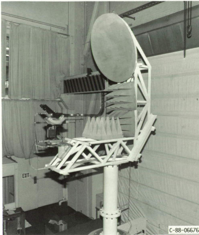
Figure 14.—Ground-based 1.4-m-diameter precision antenna.
