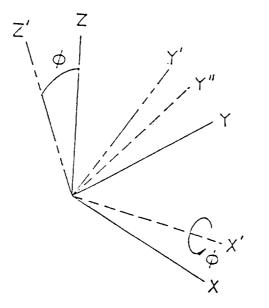
$\phi$  rotation around the X" axis to give the axis X',Y',Z'. X" and X' remain coincident.
