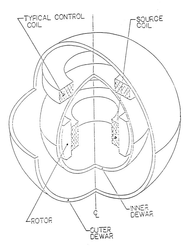
Figure 2. Advanced Slew Actuator
