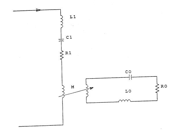
M is mutual inductance between coils; rotating coil components denoted by '0;' excited coil by '1.'
