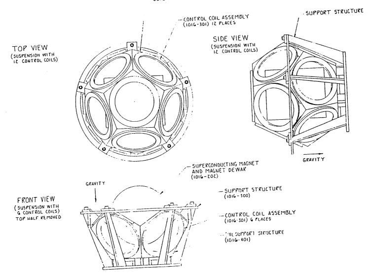
Figure 3. System Configuration
