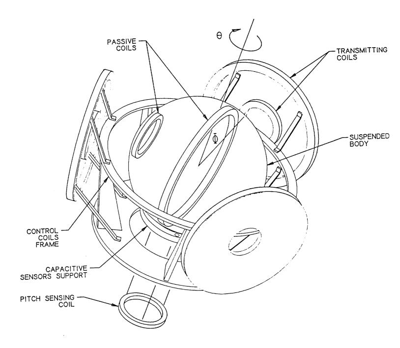
Figure 9. Position Sensing System
