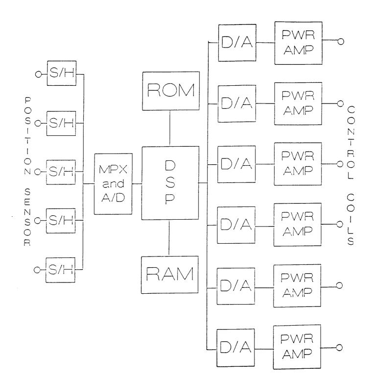
Figure 11. Electronics Block Diagram
