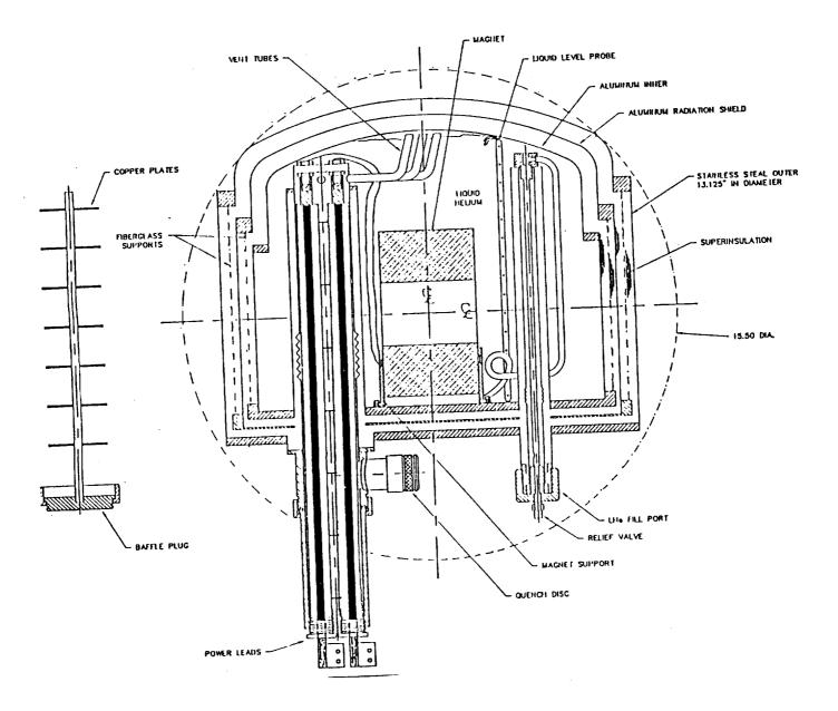
Figure 4. Magnet and Cryostat Design, Elevation View
