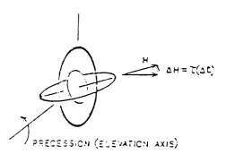
Figure 1. CMG Operating Principle
