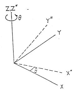
$\Theta$  rotation around the Z axis to give the intermediate axis X",Y",Z". Z and Z" remain coincident.
