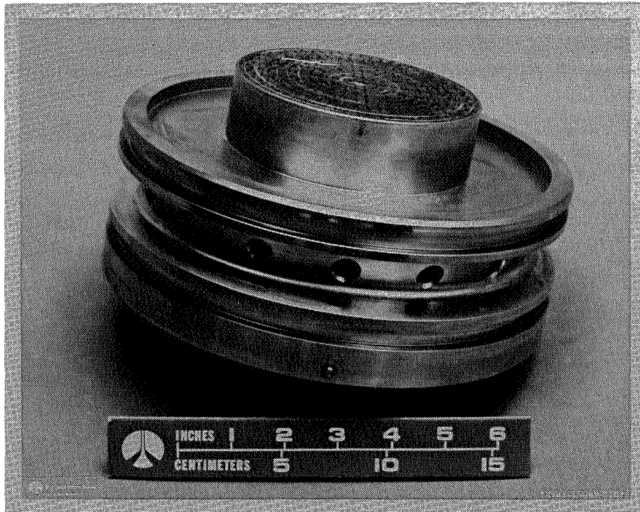
Figure 56. 5.7-Inch Canted-Fan, Like-Doublet Injector Body
